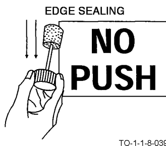
Figure 7-11. Edge Sealing
