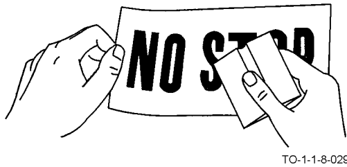
Figure 7-1. Applying Small Decal
