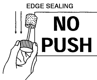
Figure 7-11. Edge Sealing
