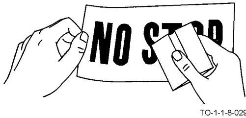
Figure 7-1. Applying Small Decal
