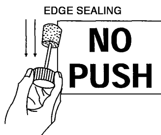
Figure 7-11. Edge Sealing
