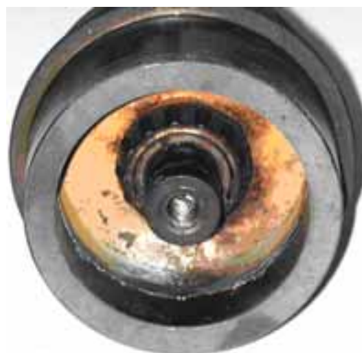
Figure 5-2. Corroded Tripod Part
