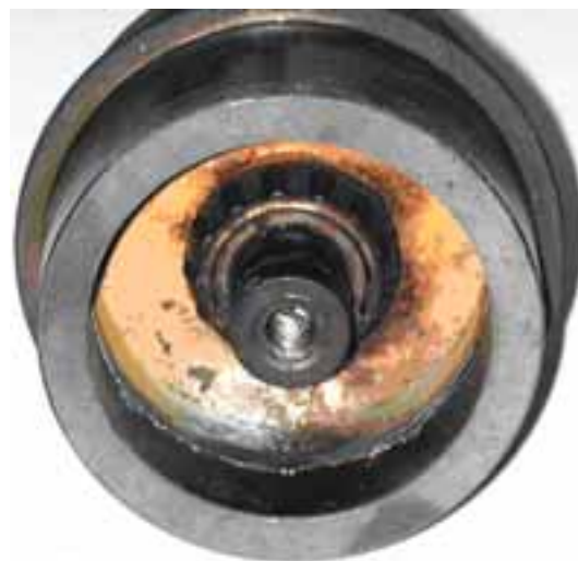
Figure 5-2. Corroded Tripod Part
