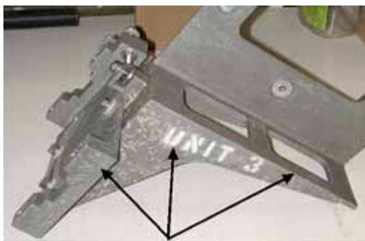
Figure 9-1. Visual Evidence of Corrosion
