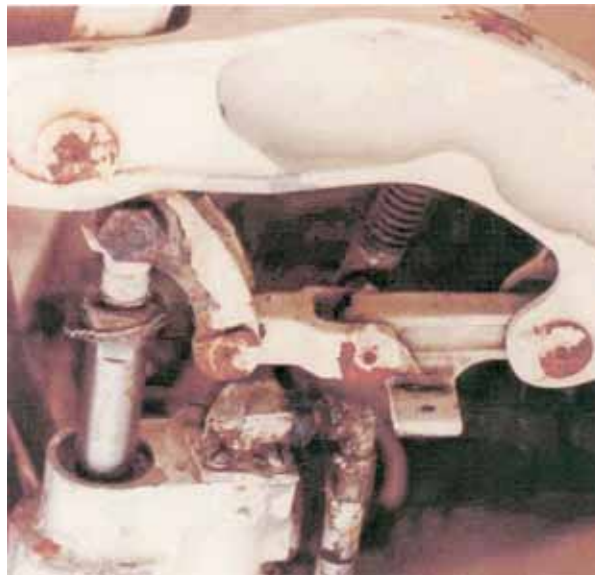
Figure 3-19. Steel Corrosion Products (Rust)
