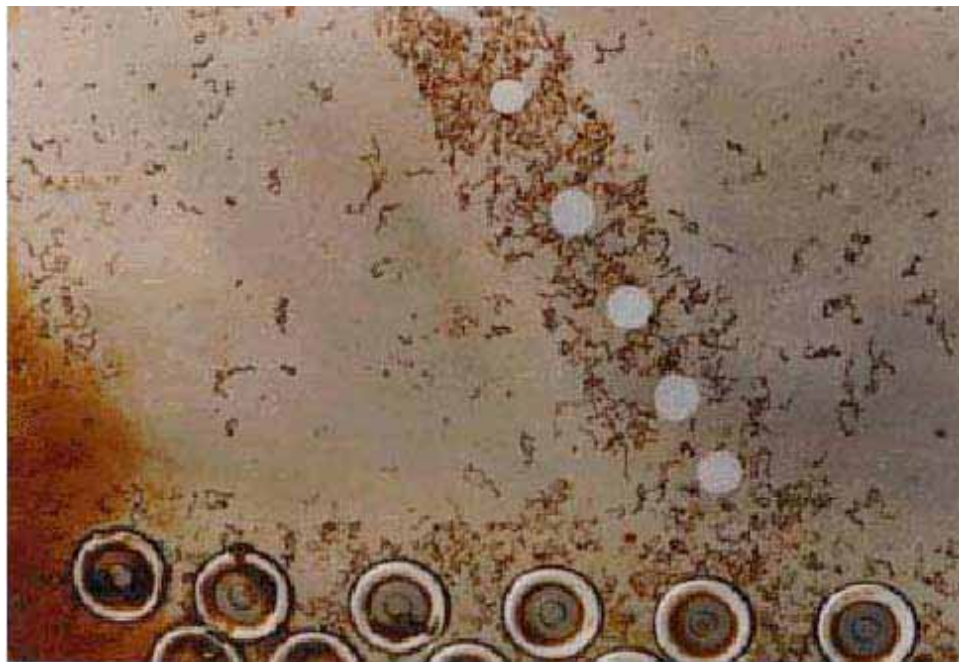
Figure 3-15. Filiform Corrosion Found Under a Paint Coating on a Magnesium Alloy Panel
