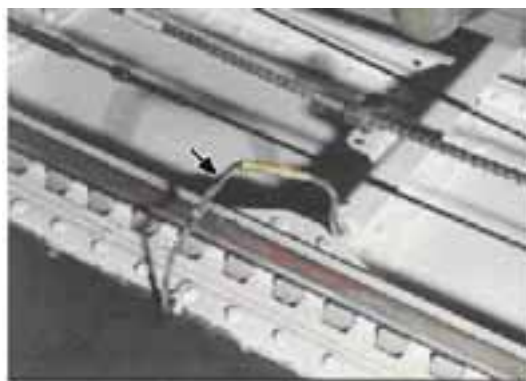
Figure 10-11. Bonding Cable Between Frame and Door
