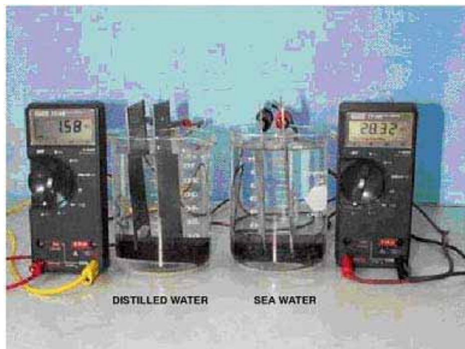
Figure 3-3. Effect of Sea Water on Galvanic Corrosion
