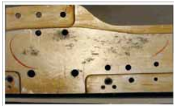
Figure 3-7. Pitting of an Aluminum Angle Assembly
