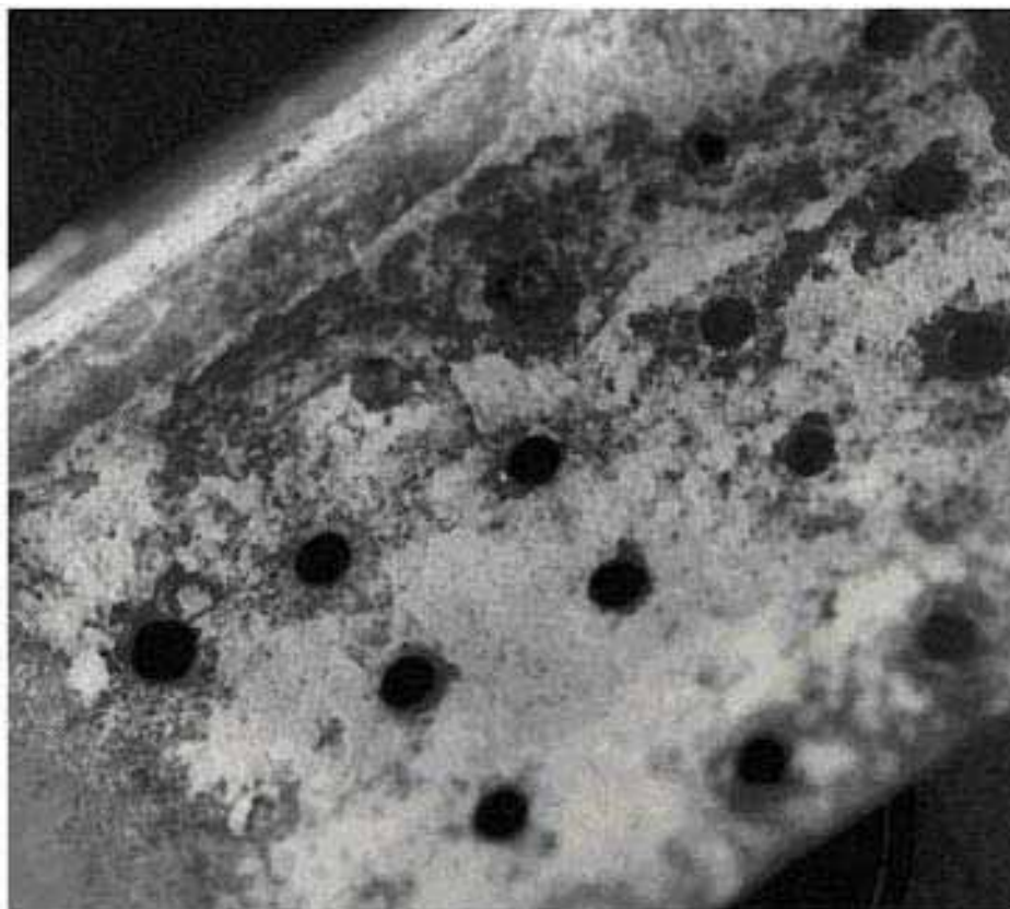
Figure 3-20. Aluminum Surface Corrosion Products
