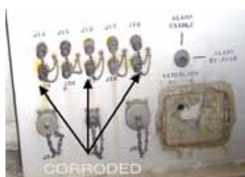
Figure 8-1. ANMST-TIV Corroded Exterior Plugs
