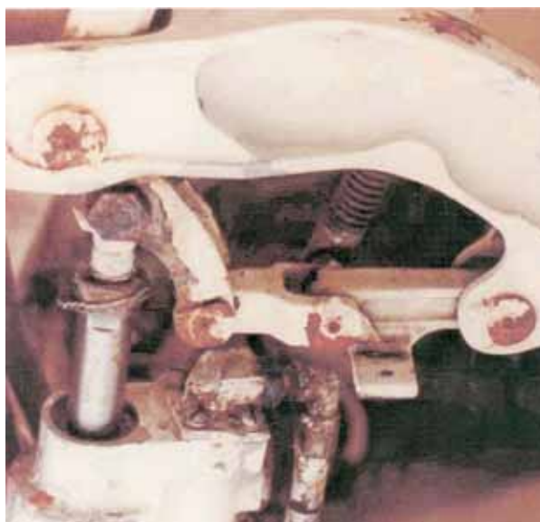
Figure 3-19. Steel Corrosion Products (Rust)
