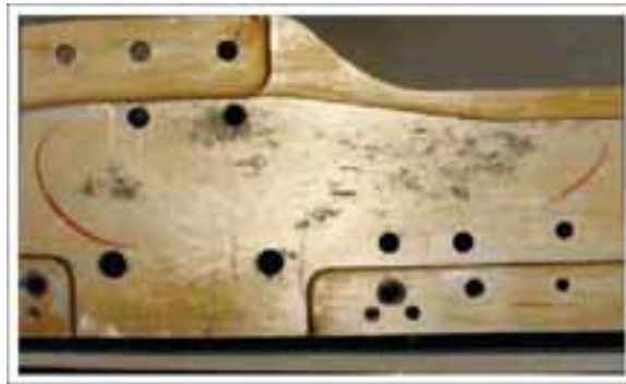
Figure 3-7. Pitting of an Aluminum Angle Assembly
