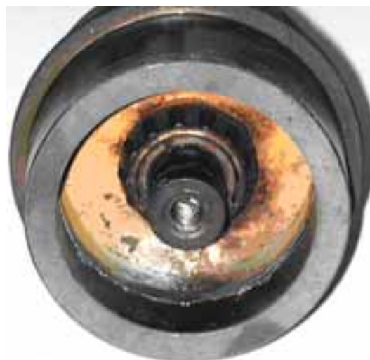
Figure 5-2. Corroded Tripod Part
