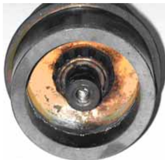
Figure 5-2. Corroded Tripod Part
