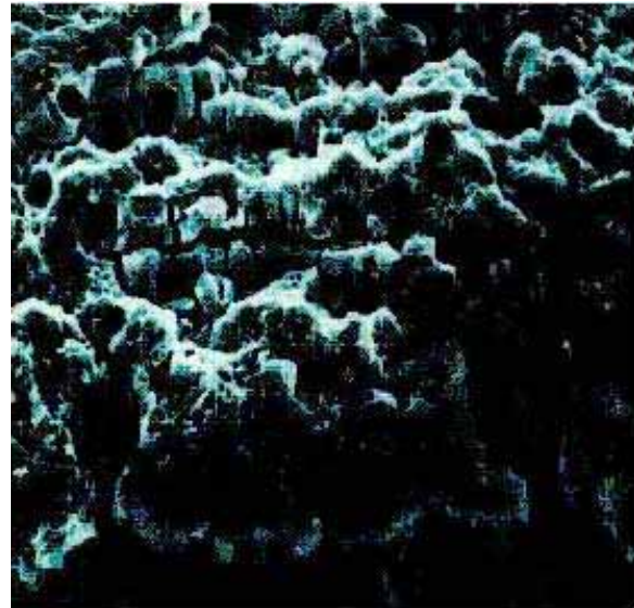
Figure 3-10. Grain Structure of a Corroding Aluminum Surface
