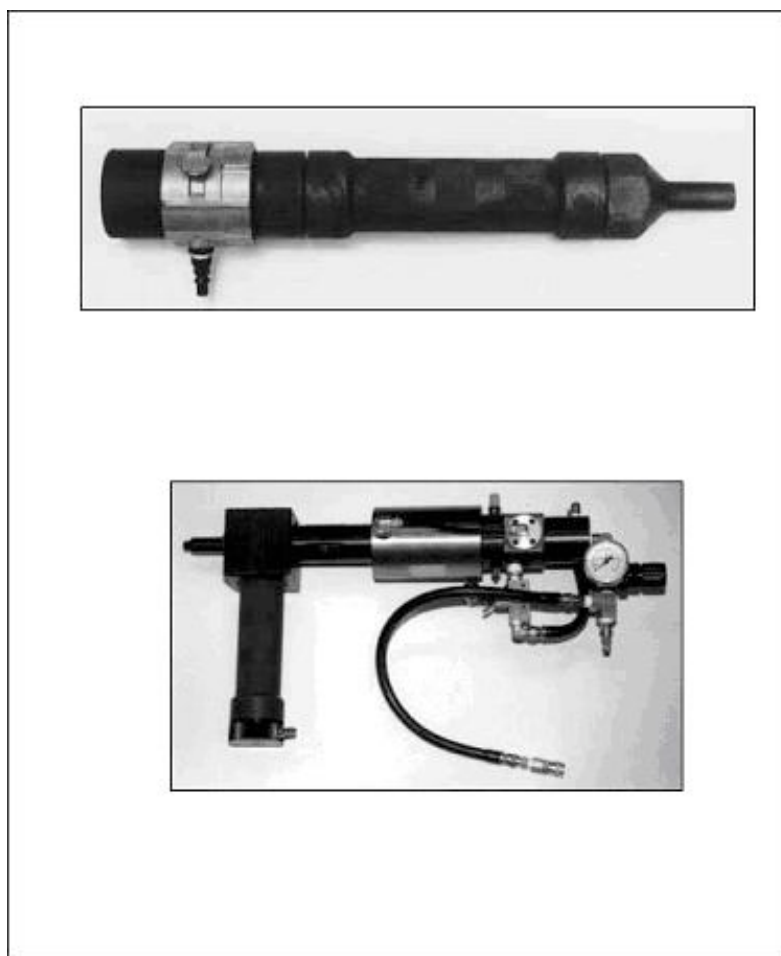
Figure 12-6. Sealant Injection Guns
