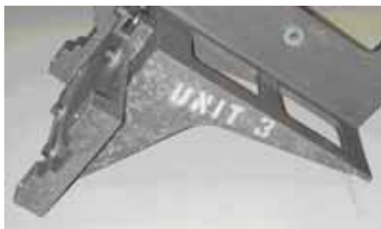
Figure 5-3. Corroded Tripod
