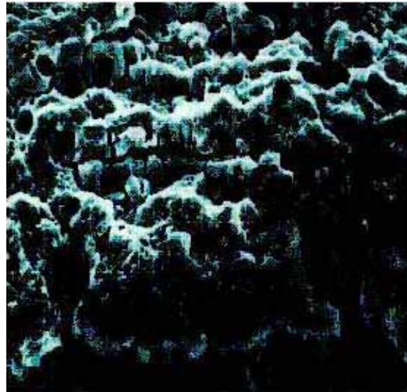
Figure 3-10. Grain Structure of a Corroding Aluminum Surface
