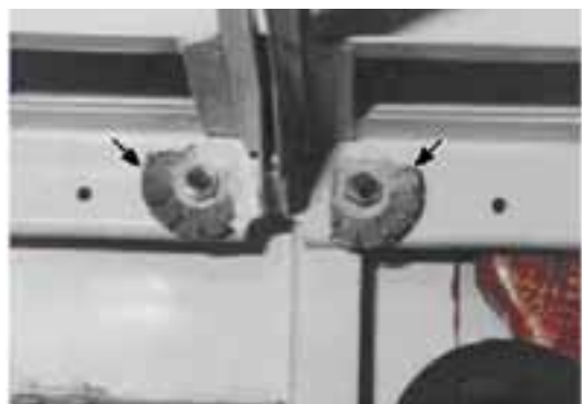
Figure 10-15. EMI Bonding Washers for Electronics
