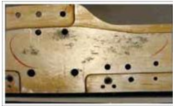
Figure 3-7. Pitting of an Aluminum Angle Assembly
