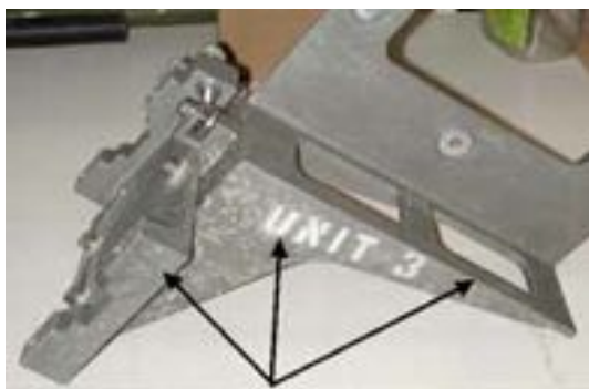
Figure 9-1. Visual Evidence of Corrosion
