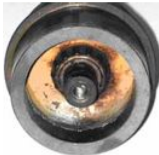
Figure 5-2. Corroded Tripod Part
