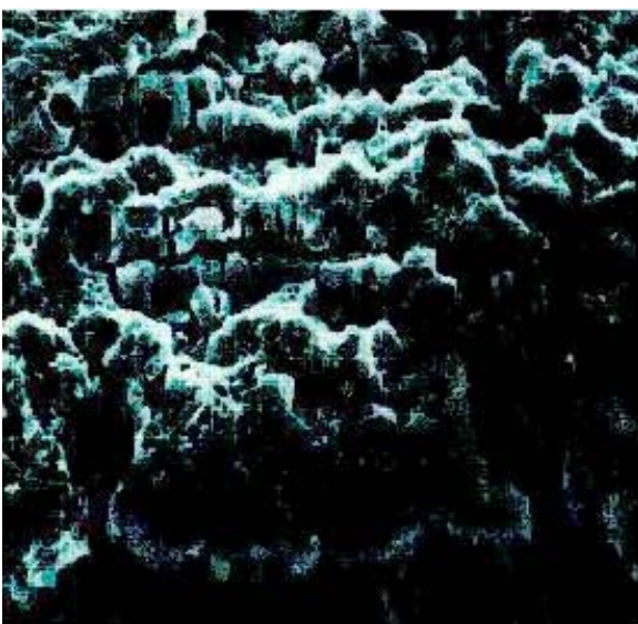
Figure 2-10. Grain Structure of a Corroding Aluminum Surface
