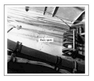
Figure 4-21. Control Cables
