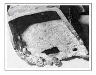
Figure 2-19. Magnesium Corrosion Products
