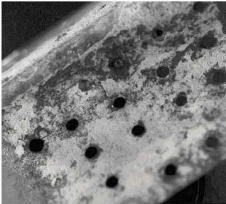
Figure 2-21. Aluminum Surface Corrosion Products
