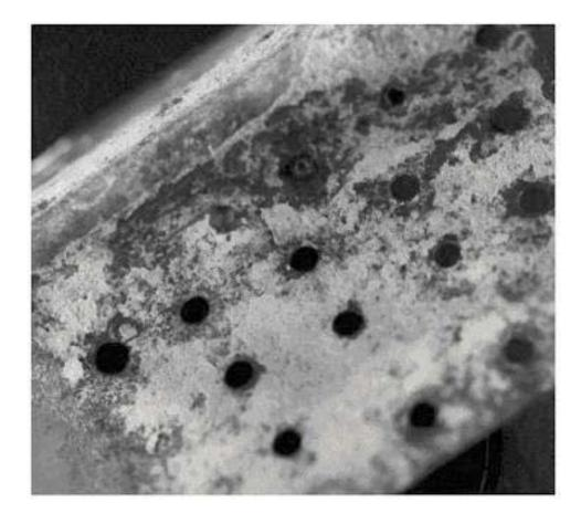
Figure 2-21. Aluminum Surface Corrosion Products
