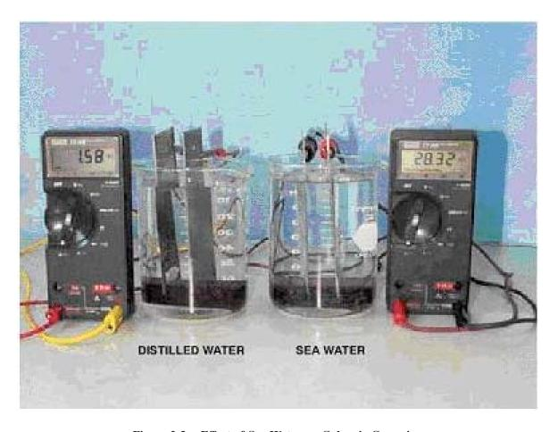
Figure 2-3. Effect of Sea Water on Galvanic Corrosion
