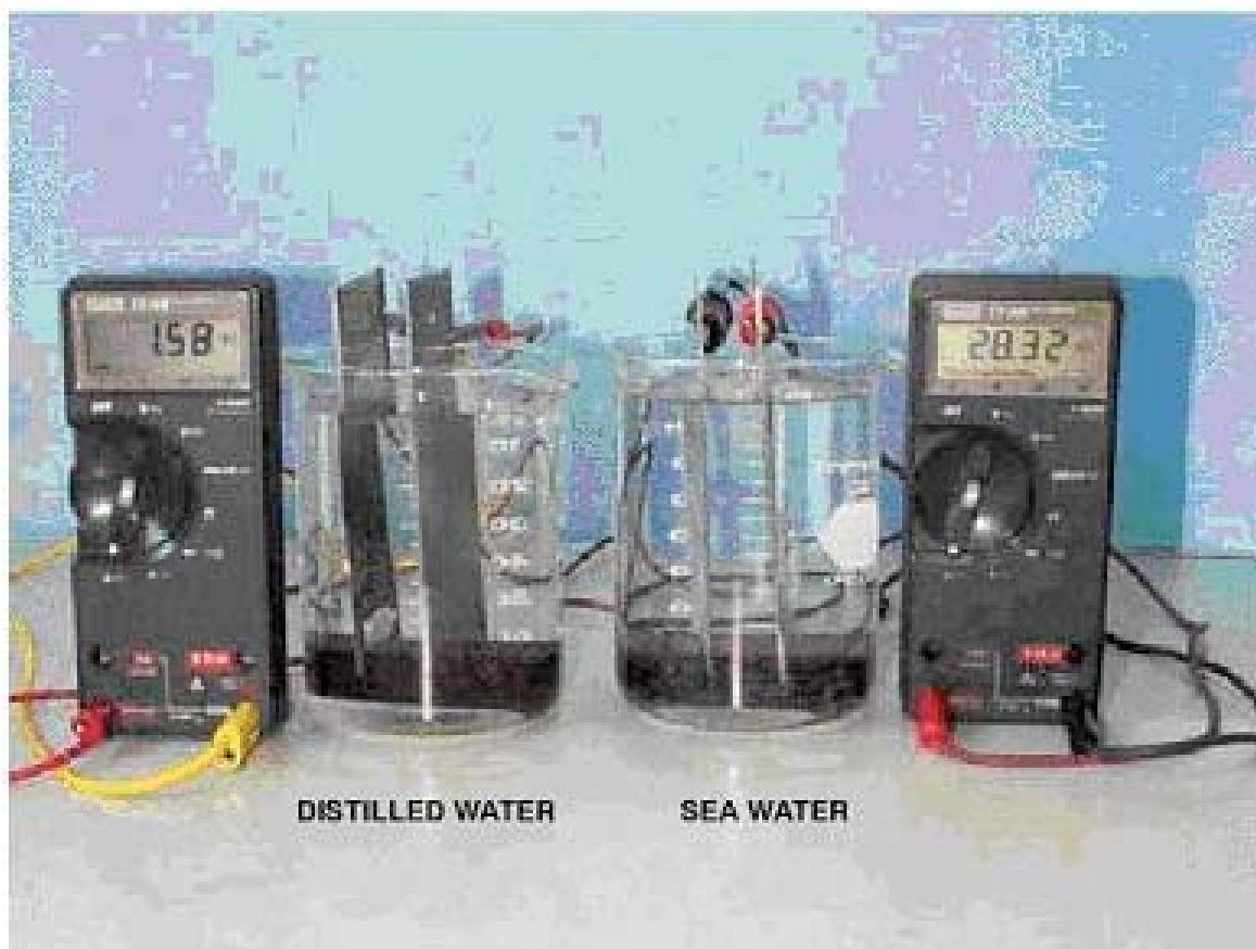
Figure 2-3. Effect of Sea Water on Galvanic Corrosion
