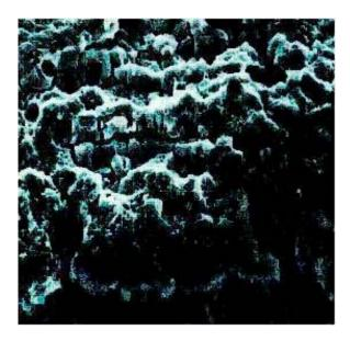
Figure 2-10. Grain Structure of a Corroding Aluminum Surface
