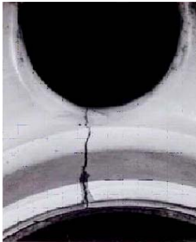
Figure 2-15. Stress Corrosion Cracking
