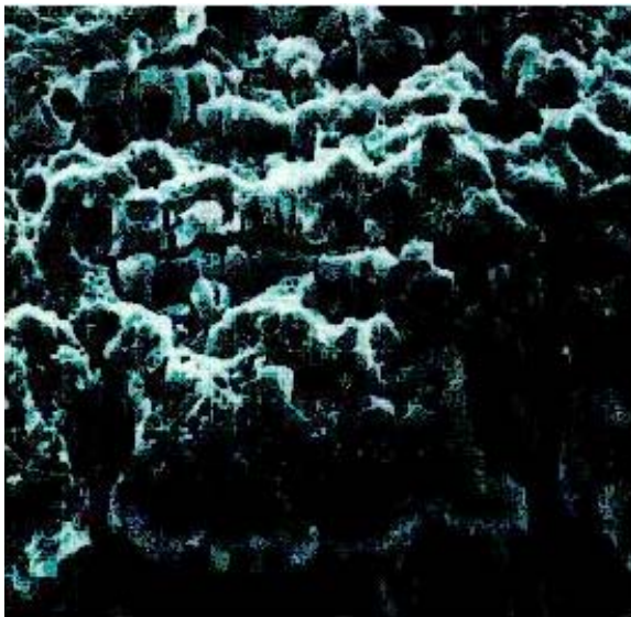
Figure 2-10. Grain Structure of a Corroding Aluminum Surface
