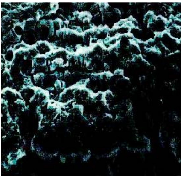
Figure 2-10. Grain Structure of a Corroding Aluminum Surface
