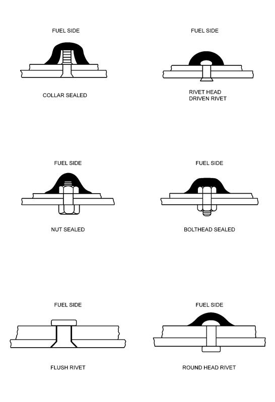
Figure 6-12. Typical Fasteners, Overcoat and Fillet
