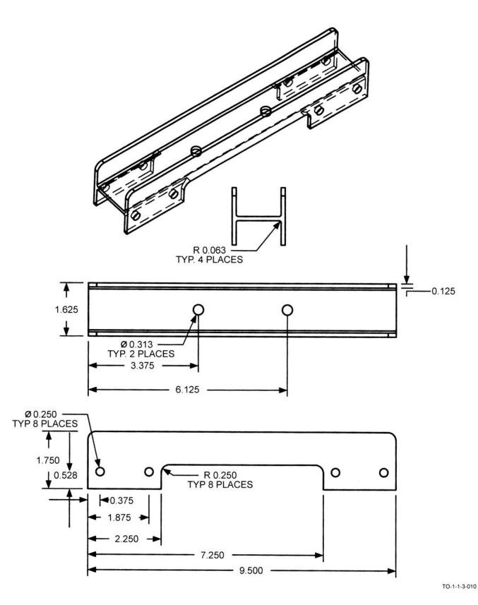
Figure 5-2. Exhaust Purge Adapter (Sheet 9)
