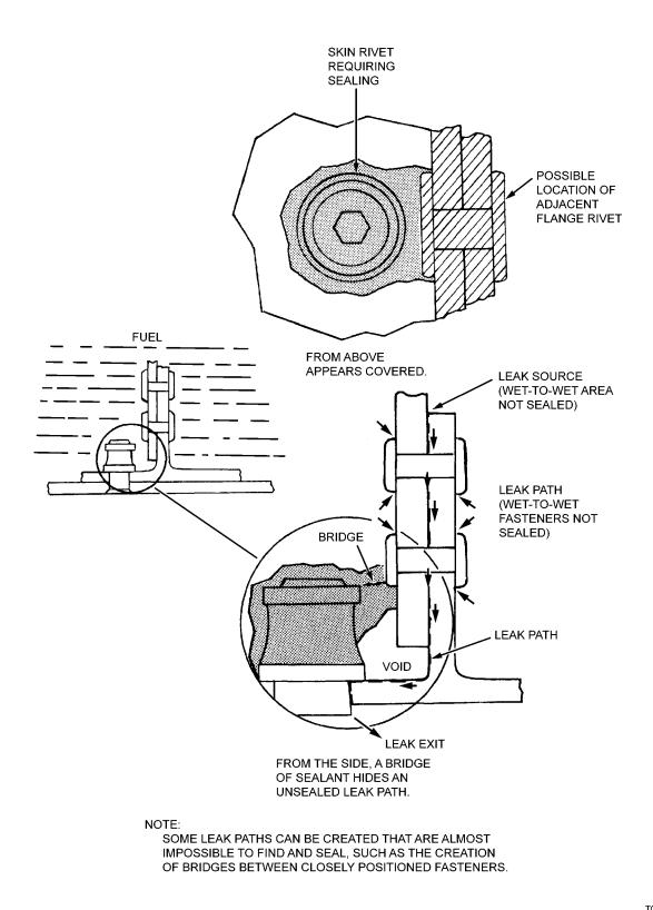
Figure 6-19. Sealant Bridging
