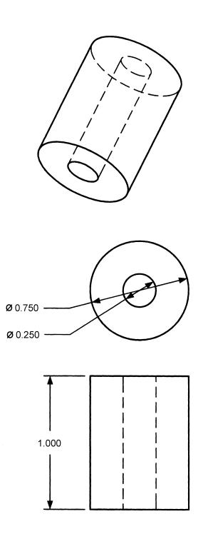
Figure 5-2. Exhaust Purge Adapter (Sheet 2)
