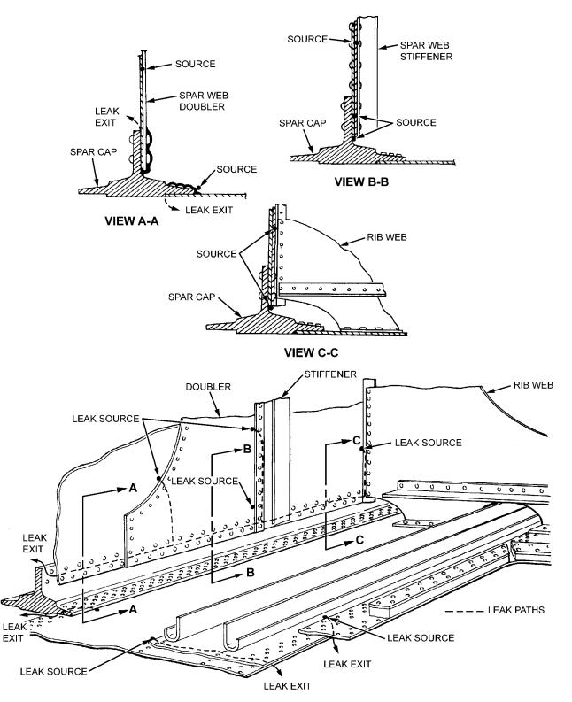
Figure 6-16. Examples of Long Leak Paths
