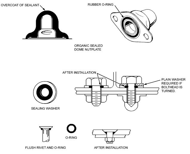
Figure 6-11. Typical Fastener Seal
