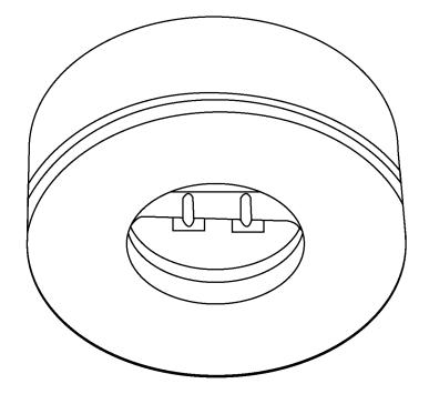
Figure 5-2. Exhaust Purge Adapter (Sheet 12)
