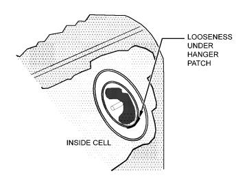
Figure 9-13. Looseness Under Hanger Fitting
