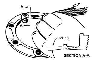
Figure 9-29. Fitting Flange Break
