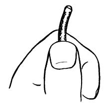
4. ROUNDED END OF LACING LINE PROPERLY PREPARED FOR USE.
