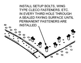
Figure 6-32. Faying Surface Seal Assembly
