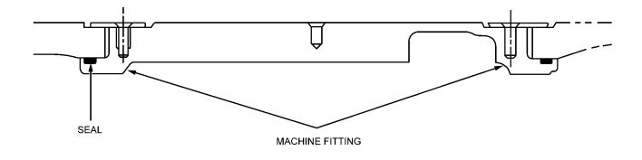
Figure 6-13. Machine Fitted Plug-Type Access Door for Attaching Screws
