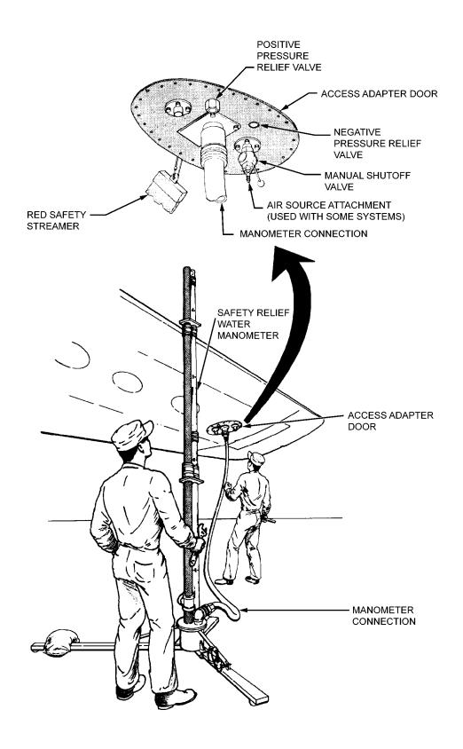
Figure 6-21. Pressure Test Method
