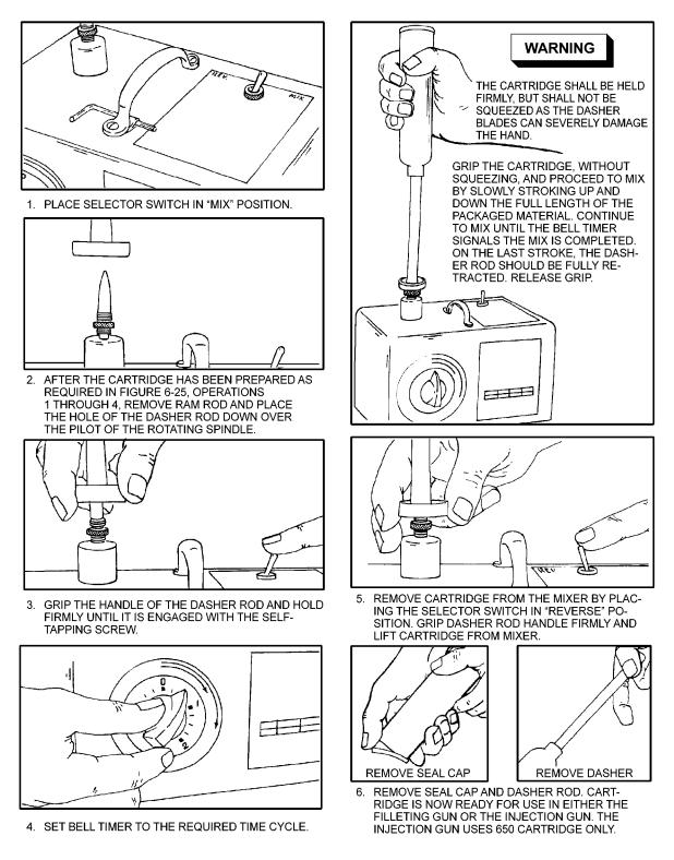
Figure 6-26. Machine Mixing of Cartridges
