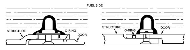
Figure 6-9. O-Ring Seal
