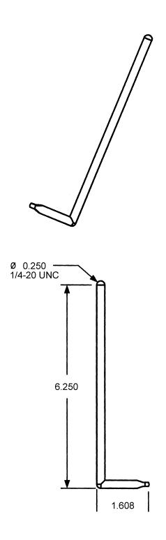
Figure 5-2. Exhaust Purge Adapter (Sheet 3)
