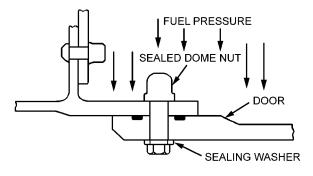
Figure 6-7. Direct Seal Door
