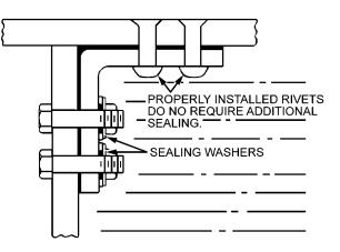
Figure 6-5. Structural Adhesive Sealing
