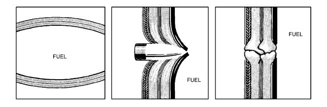
Figure 9-1. Projectile Sealing Action
