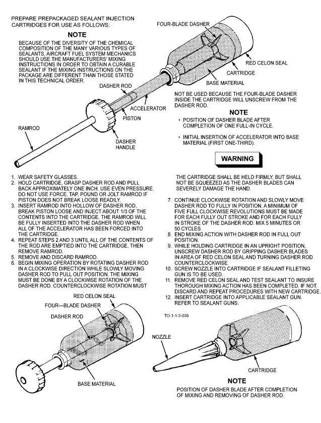
Figure 6-25. Hand Mixing of Sealant Kit
