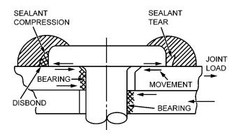
Figure 6-17. Fastener Movement on Oversize Hole
