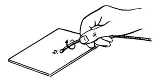
2. ROLL MELTED END ON CARDBOARD OR ANY FLAT SURFACE TO REMOVE EXCESS NYLON AND TO FORM SHARP TIP ON END OF LINE.
