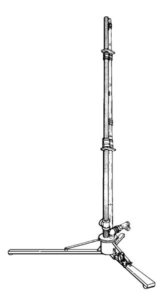
Figure 8-2. Water Manometer
