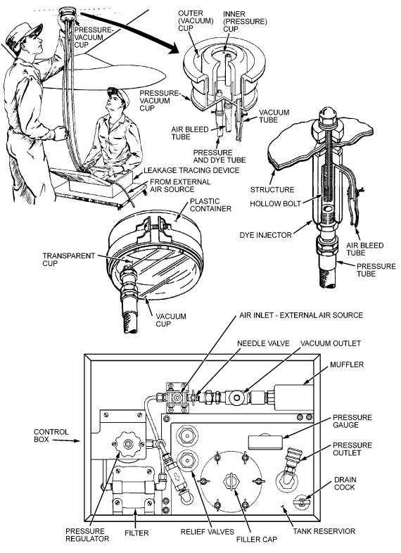
Figure 6-23. Dye Injection Method
