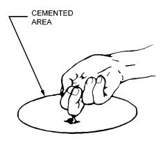
Figure 9-18. Knuckle Test
