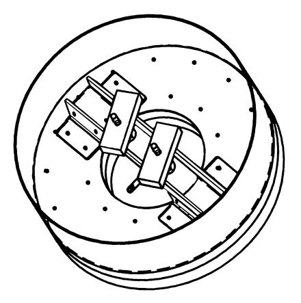
Figure 5-2. Exhaust Purge Adapter (Sheet 8)
