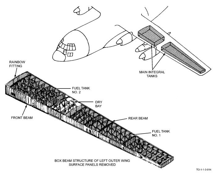
Figure 6-1. Typical Integral Fuel Tanks
