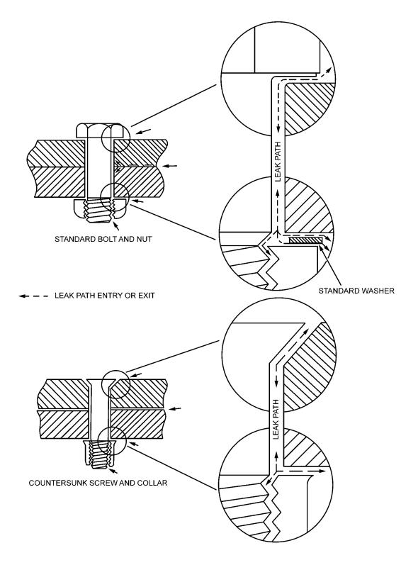
Figure 6-15. Fasteners Leaks
