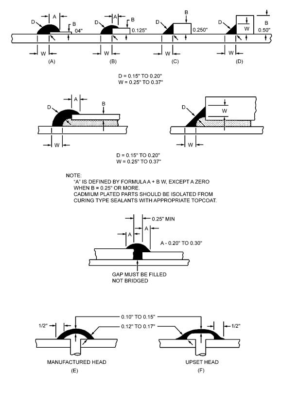
Figure 6-30. Typical Fillet Dimensions
