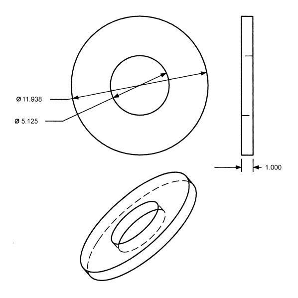
Figure 5-2. Exhaust Purge Adapter (Sheet 5)
