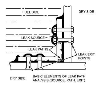
Figure 6-14. Leak Path Analysis
