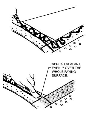
Figure 6-31. Applications of Faying Surface Sealant
