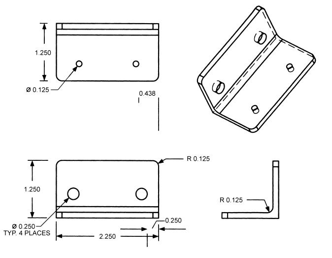
Figure 5-2. Exhaust Purge Adapter (Sheet 10)
