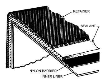
Figure 9-2. Self-Sealing
