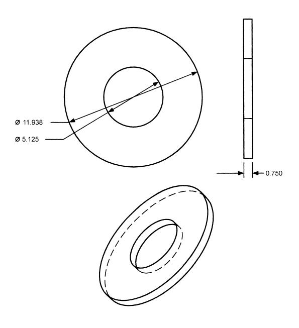
Figure 5-2. Exhaust Purge Adapter (Sheet 6)
