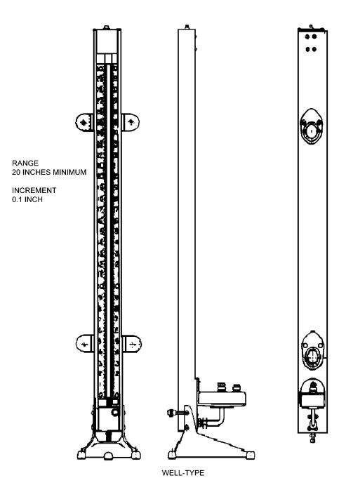
Figure 8-4. Typical Well-Type Manometer
