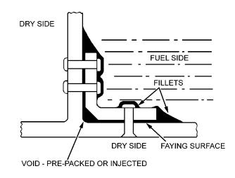
Figure 6-2. Curing Sealant Design
