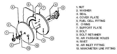
Figure 9-32. Fuel Cell Fitting Leak Test Cover Plate
