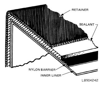
Figure 9-2. Self-Sealing
