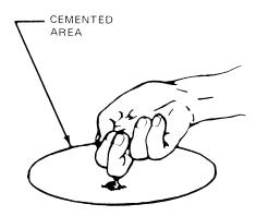
Figure 9-18. Knuckle Test
