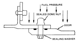
Figure 6-7. Direct Seal Door
