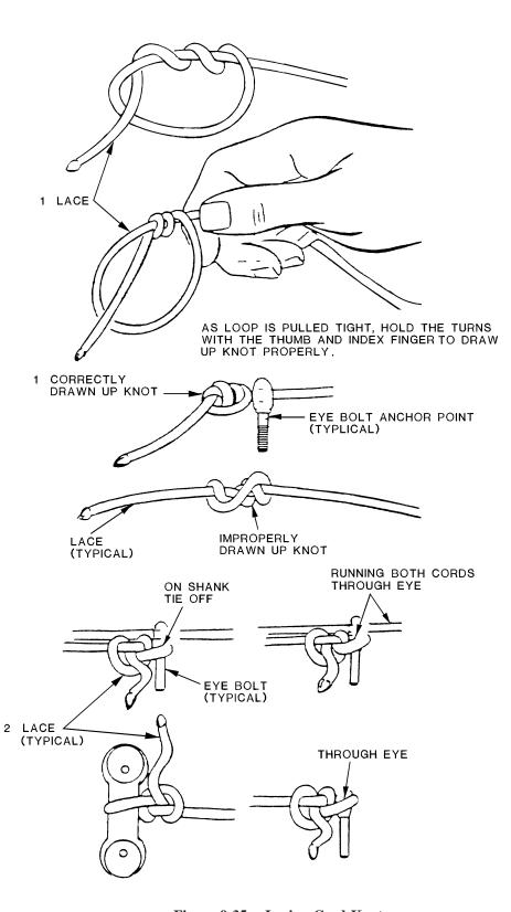
Figure 9-35. Lacing Cord Knots
