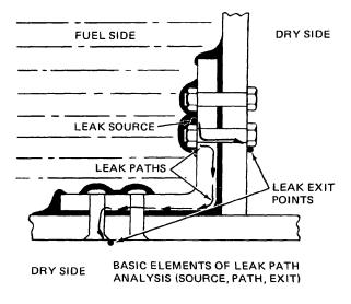
Figure 6-14. Leak Path Analysis
