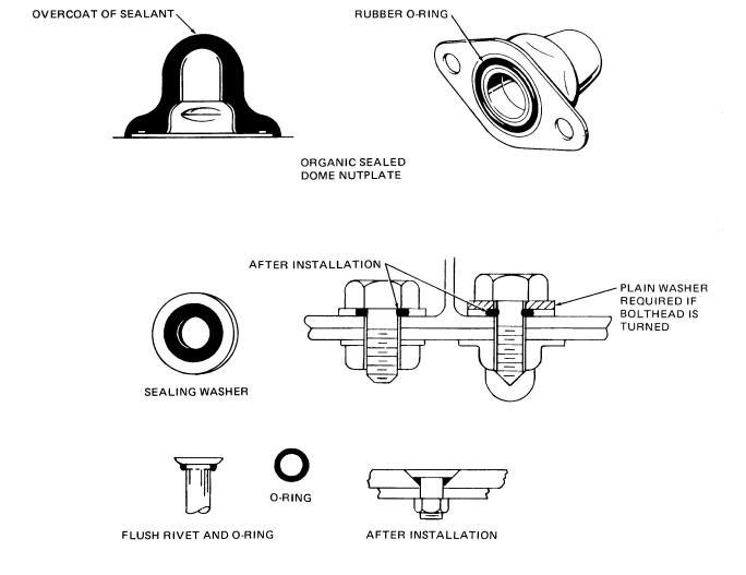
Figure 6-11. Typical Fastener Seal
