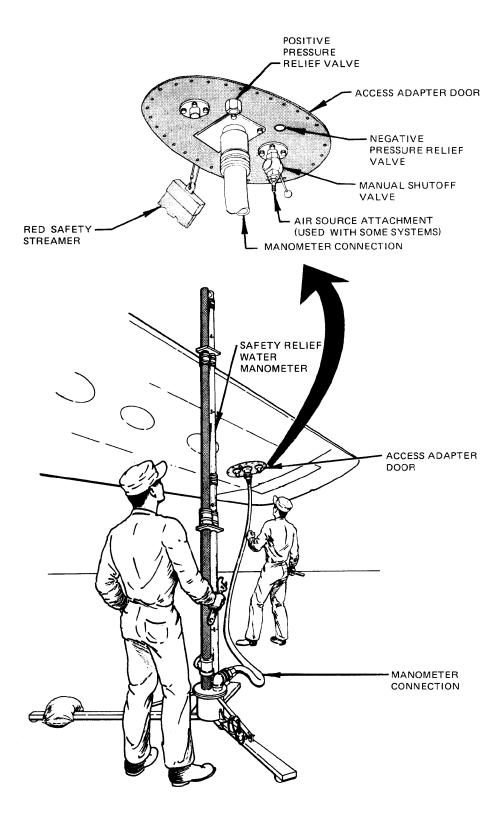
Figure 6-21. Pressure Test Method
