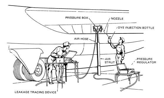
Figure 6-24. Use of Pressure Box for Dye Injection
