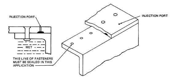
Figure 6-4. Typical Locations of Grooves/Channels (Sheet 1 of 2)
