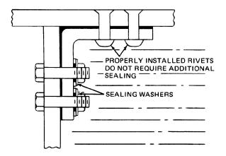
Figure 6-5. Structural Adhesive Sealing
