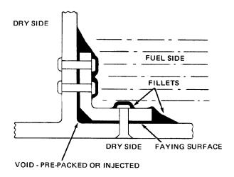
Figure 6-2. Curing Sealant Design
