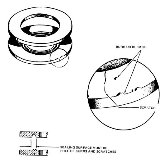
Figure 9-12. O-Ring Fitting Inspection
