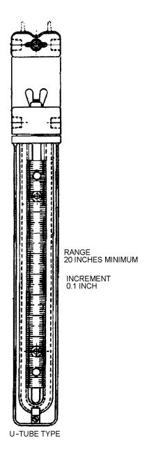
Figure 8-4. Typical U-Tube-Type Manometer
