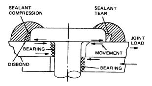
Figure 6-17. Fastener Movement on Oversize Hole
