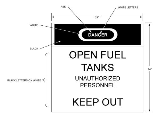
Figure 8-1. Marking of Fuel System Repair Area
