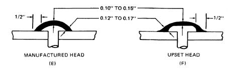
Figure 6-30. Typical Fillet Dimensions
