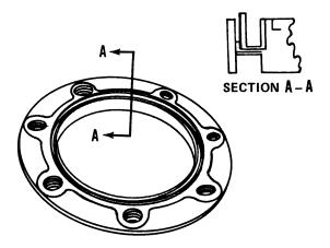
Figure 9-30. Retainer Ring Installation
