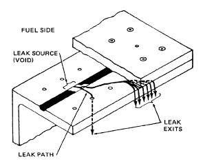
Figure 6-27. Void in Non-Curing Sealant Groove
