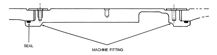
Figure 6-13. Machine Fitted Plug-Type Access Door for Attaching
