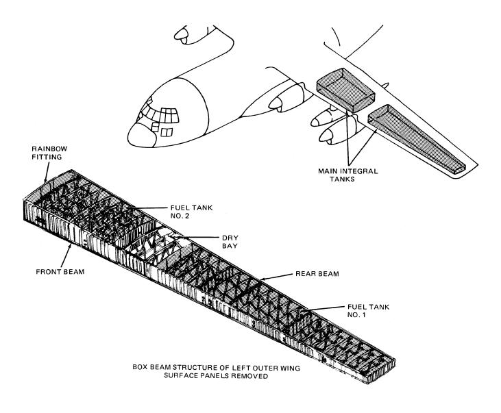
Figure 6-1. Typical Integral Fuel Tanks
