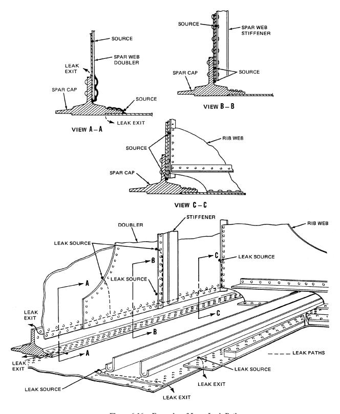
Figure 6-16. Examples of Long Leak Paths
