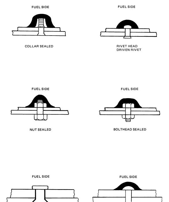
Figure 6-12. Typical Fasteners, Overcoat and Fillet
