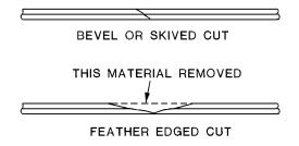
Figure 9-21. Sectional Views of Corner Patch
