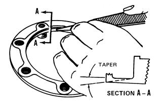
Figure 9-29. Fitting Flange Break
