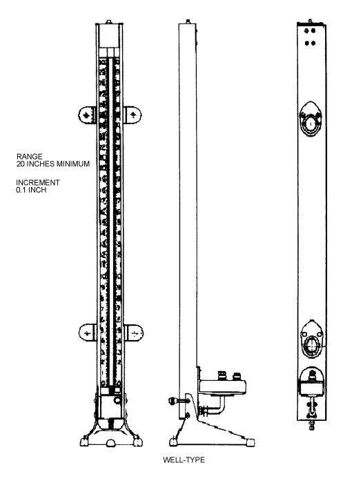
Figure 8-5. Typical Well-Type Manometer
