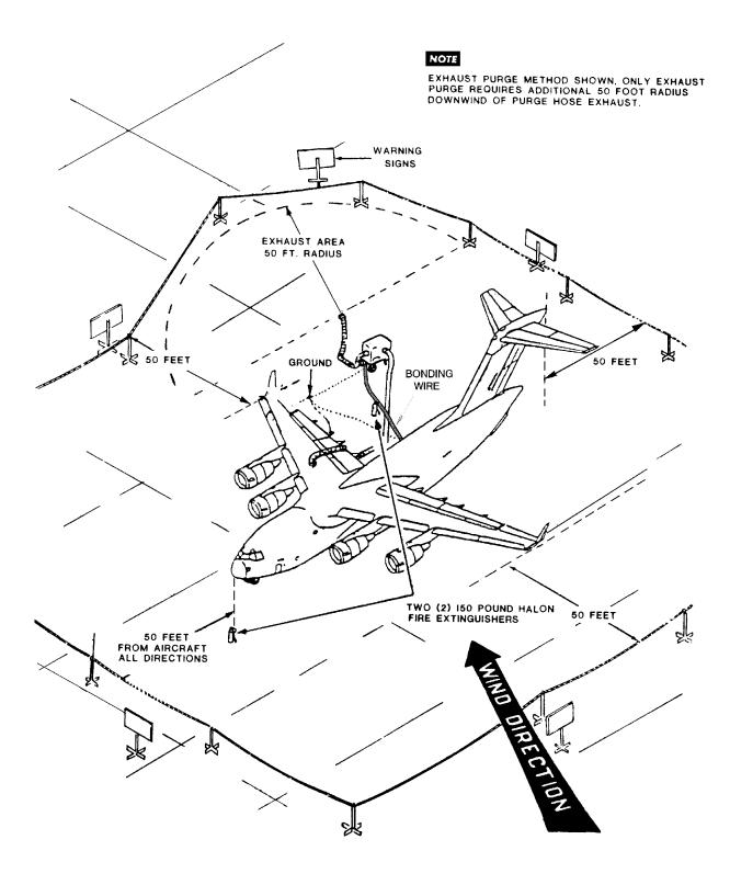
Figure 5-1. Typical Combination Purge in Open Repair Area
