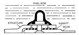
Figure 6-8. Flat Gasket Seal
