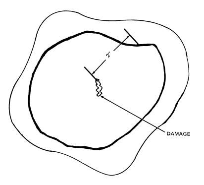
Figure 9-16. Marking Area To Be Repaired
