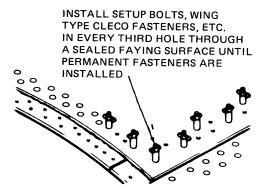
Figure 6-32. Faying Surface Seal Assembly
