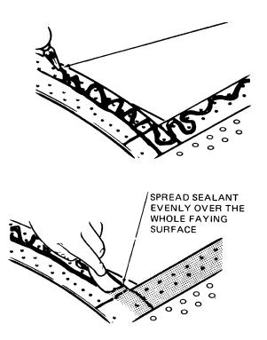
Figure 6-31. Applications of Faying Surface Sealant
