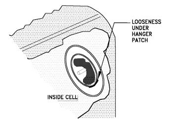
Figure 9-13. Loosen Under Hanger Fitting
