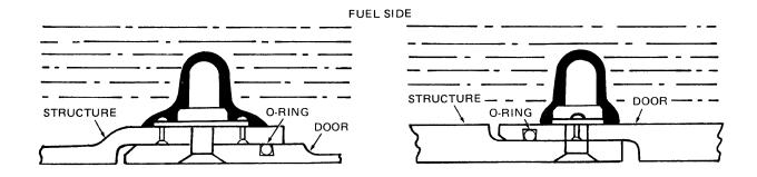
Figure 6-9. O-Ring Seal
