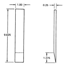
Figure 8-7. Typical Hand Scraper
