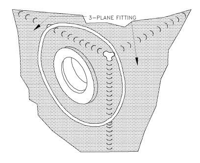
Figure 9-15. Three-Plane Fitting
