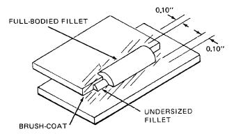
Figure 6-28. Two Bead Fillet
