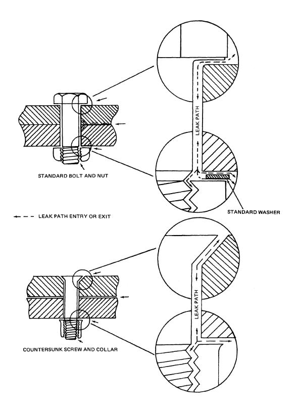
Figure 6-15. Fasteners Leaks
