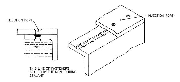
Figure 6-4. Typical Locations of Grooves/Channels (Sheet 2)
