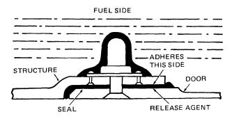
Figure 6-10. Formed-In-Place Seal
