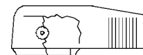
ONE CRACK EXTENDING ABOVE SET SCREW NOT PERMISSIBLE. ONE CRACK BELOW SET SCREW PERMISSIBLE.
