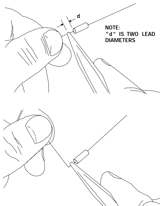
Figure 3-15. Lead Bending Method
