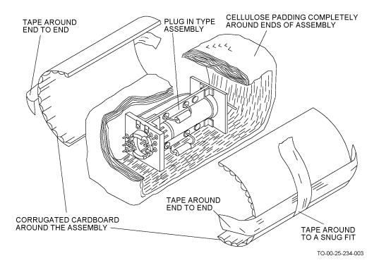
Figure 2-3. Plug-In Type Electronic Assembly, Protective Packaging
