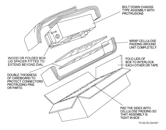
Figure 2-1. Chassis-Type Electronic Assembly, Protective Packaging
