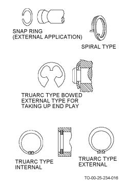
Figure 4-13. Typical Retaining Rings
