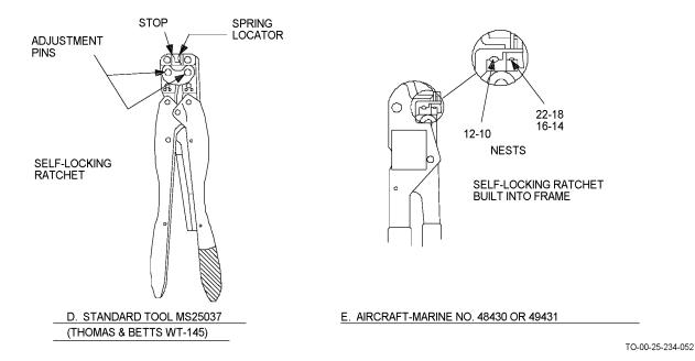
Figure 4-49. Hand Crimping Tools for Pre-Insulated Terminals
