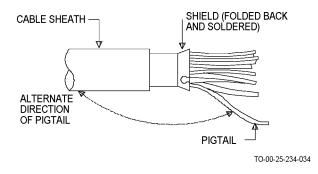
Figure 4-31. Soldered On Pigtail Preparation
