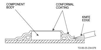
Figure 6-5. Removing Polyurethane Coating from Lead
