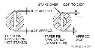
Figure 4-4. Application of Tapered Pins
