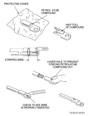
Figure 4-48. Inserting Aluminum Wire Into Aluminum Terminal Lugs
