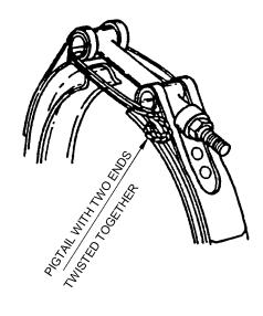
Figure 4-20. V-Band Coupling Safety Wiring Techniques
