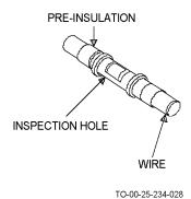
Figure 4-25. Pre-Insulated Permanent Copper Splices
