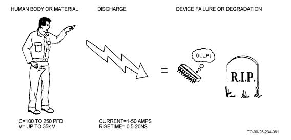
Figure 7-1. Reasons for Device Failure Due to ESD
