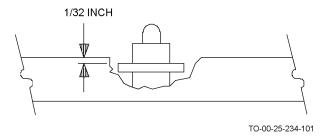
Figure 8-6. Typical Excavated Plug
