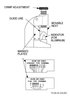
Figure 4-50. Hand Crimping Tool, Aluminum Terminals
