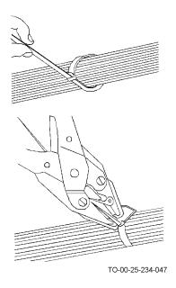
Figure 4-44. Nylon Strapped Spot Tie
