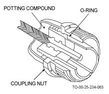
Figure 4-60. Installation of O-Ring on Potted Connector
