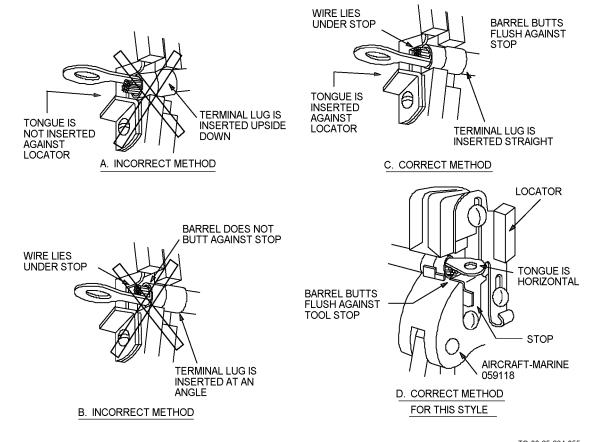
Figure 4-52. Inserting Terminal Lug Into Hand Tool
