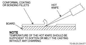
Figure 6-6. Removing Polyurethane Coating or Fillets
