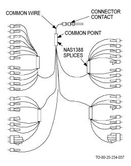
Figure 4-34. Typical Cascading Pigtails
