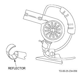
Figure 4-56. Electric Hot-Air Gun
