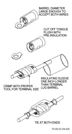
Figure 4-26. Terminal Lug Barrel Splice
