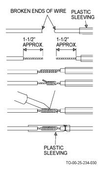
Figure 4-27. Splicing Broken Wire by Soldering
