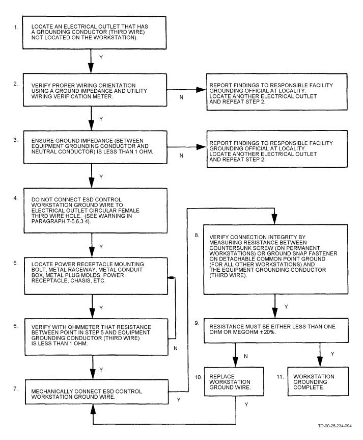
Figure 7-14. Flow Chart for ESD Control Workstation Grounding
