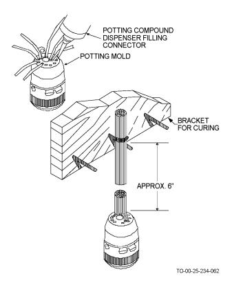
Figure 4-59. Filling and Curing Potted Connector
