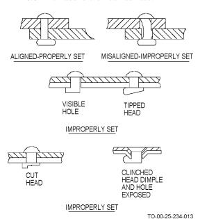
Figure 4-10. Properly and Improperly Set Rivets
