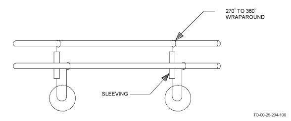
Figure 8-5. Buss Wire Connection
