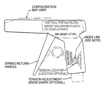
Figure 4-42. MS90387 Adjustable Hand Tools for Installing Self-Clinching Plastic Tiedown Straps
