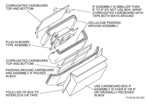
Figure 2-2. Circuit Board-Type Electronic Assembly, Protective Packaging
