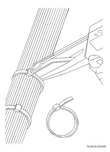
Figure 4-41. Installing Self-Clinching Plastic Cable Straps
