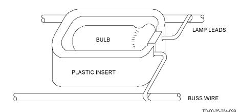
Figure 8-4. Typical Bulb Insert
