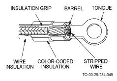
Figure 4-46. Pre-Insulated Terminal Lug Cutaway
