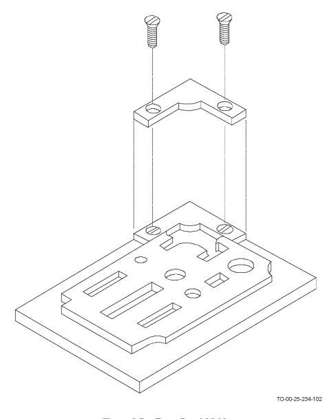
Figure 8-7. Front Panel Mold
