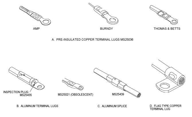
Figure 4-45. Solderless Terminal Lugs
