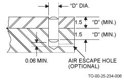
Figure 4-3. Application of Dowel Pin
