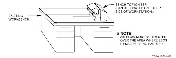
Figure 7-6. Bench Top Ionizer Positioning
