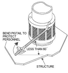
Figure 4-22. Safety Wiring AN Connector to Structure
