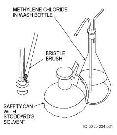
Figure 4-58. Cleaning Connector Prior to Potting
