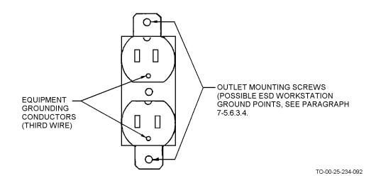
Figure 7-12. Typical Electrical AC Outlet
