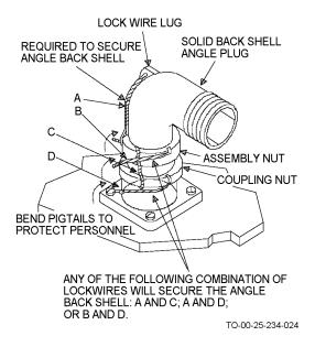
Figure 4-21. Safety Wiring AN Connectors
