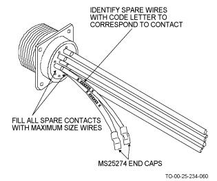
Figure 4-57. Spare Wires for Potted Connector
