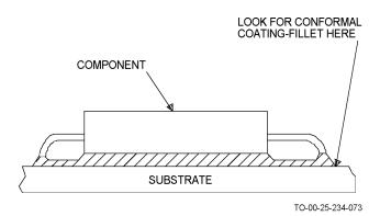
Figure 6-2. Conformal Coating Fillet
