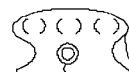
ONE CRACK EXTENDING ABOVE SET SCREW NOT PERMISSIBLE. ONE CRACK BELOW SET SCREW PERMISSIBLE.
