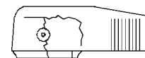
ONE CRACK EXTENDING ABOVE SET SCREW NOT PERMISSIBLE. ONE CRACK BELOW SET SCREW PERMISSIBLE.
