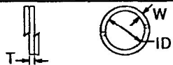
Chart 2B-2 DOUBLE-TURN BACKUP RINGS FOR USE GLAND O-RINGS IN MIL-H-5606 AND MIL-H-83282 HYDRAULIC FLUIDS
