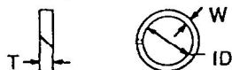
Chart 2B-1 SINGLE-TURN BACKUP RINGS FOR USE WITH GLAND O-RINGS IN MIL-H-5606 AND MIL-H-83282 HYDRAULIC FLUIDS (CONTD)
