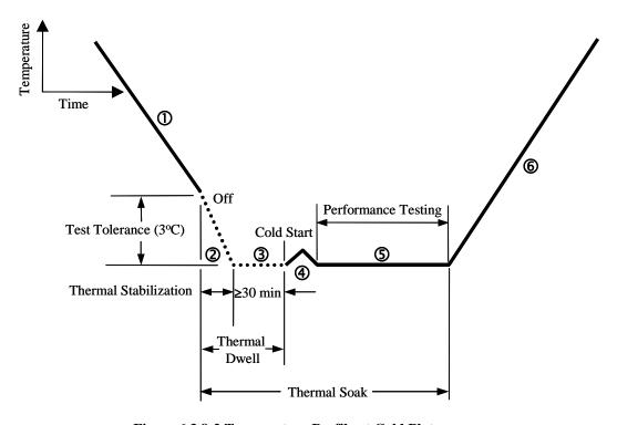
Figure 6.3.8-2 Temperature Profile at Cold Plateau
