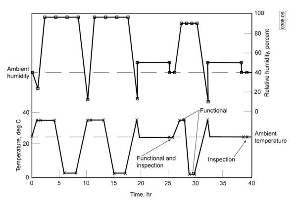
Figure 6.3.10-1 Humidity Test Time Line
