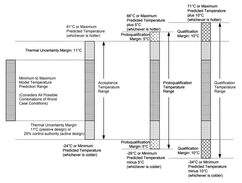
Figure 6.3.8-3. Unit Test Temperature Ranges and Margins
