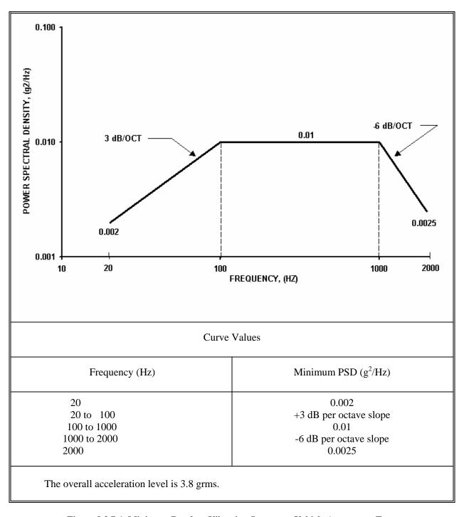
Figure 8.3.7-1 Minimum Random Vibration Spectrum, Vehicle Acceptance Tests
