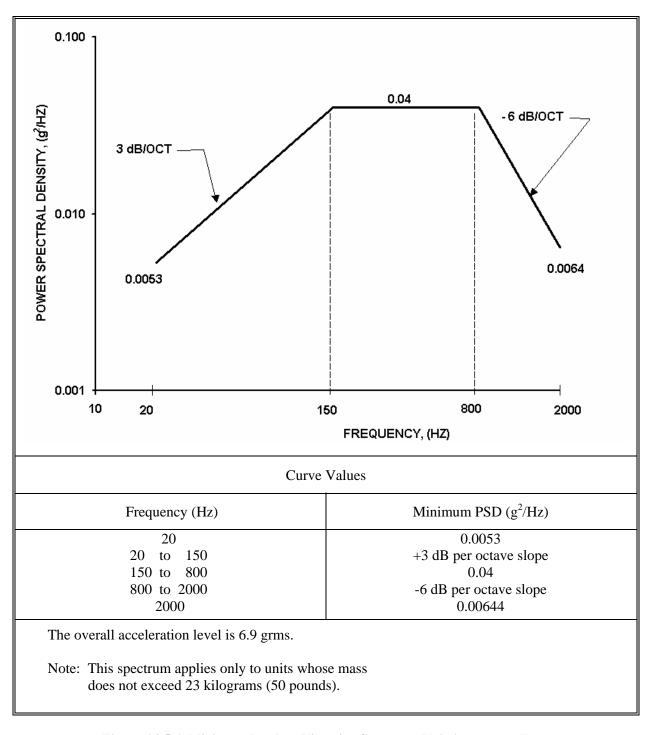
Figure 6.3.5-1 Minimum Random Vibration Spectrum, Unit Acceptance Tests
