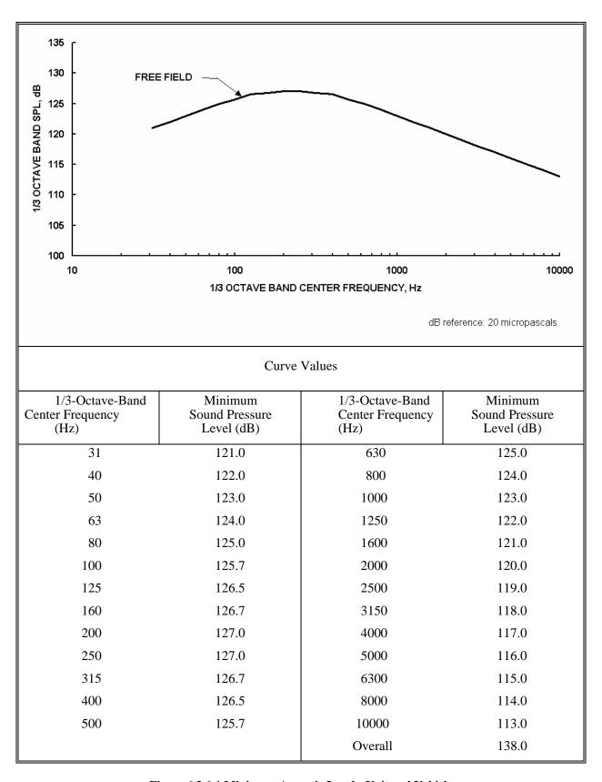
Figure 6.3.6-1 Minimum Acoustic Levels, Unit and Vehicle
