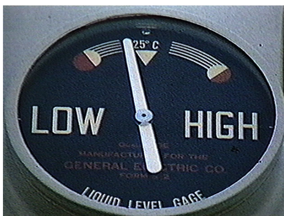
Picture 3-9 Liquid-level gauge
