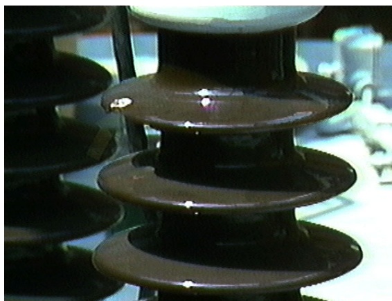
Picture 7-2 Correctable bushing chip
