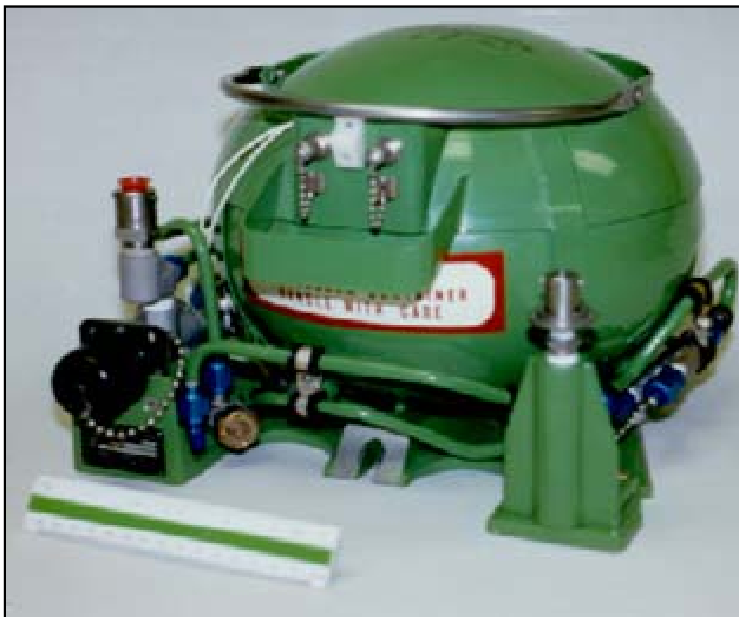
Figure A-1. F-15A-D Legacy Liquid Oxygen (LOX) Converter.
