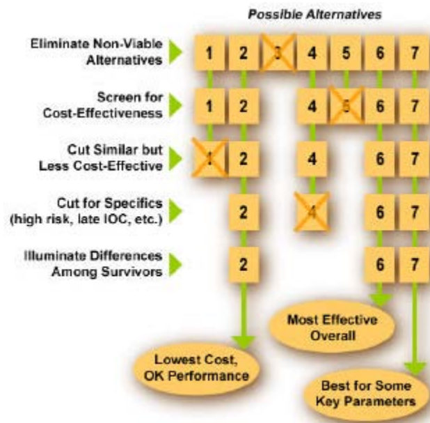
Figure 5-1: Eliminating Alternatives in an AoA
