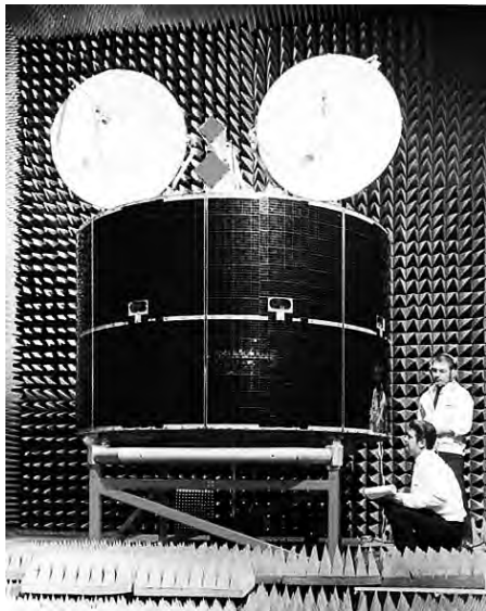
Figure 22-6. Spacecraft with body-mounted solar array. (Air Force photo)
