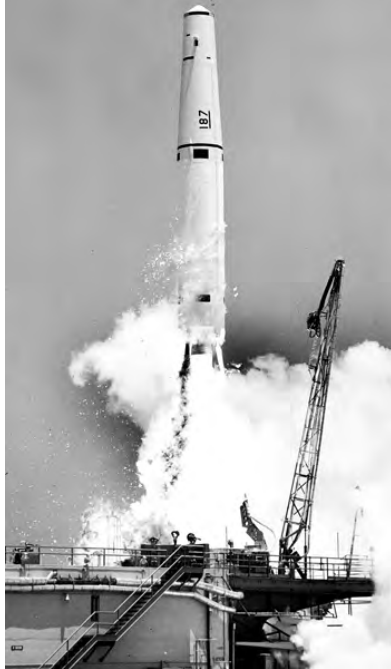
Figure 18-3. A test Thor takes flight at Cape Canaveral, FL, on 5 December 1959. The small particles falling away from the rocket are ice formed from frozen condensation on the outside of the chilled liquid oxygen tank. (USAF photo)
