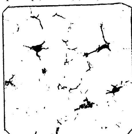
Scale of a microstructure with residual microporosity (six levels) (x100) b
