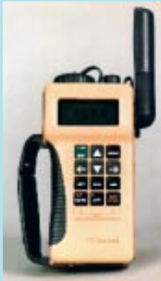
US Military Precision Lightweight GPS Receiver
