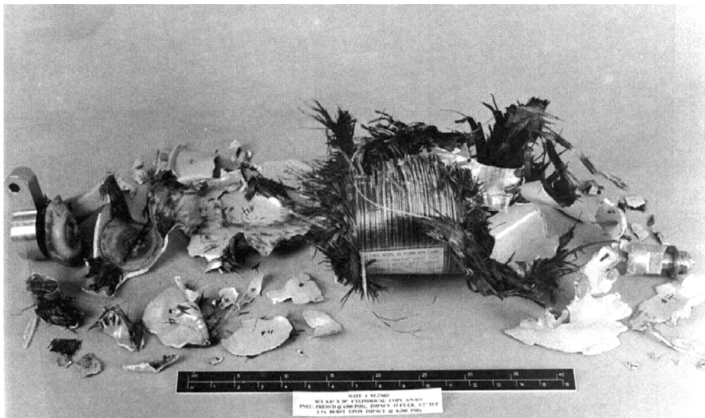
Figure B-4. Vessel remnants after pneumatic burst at impact, Test S-33.
