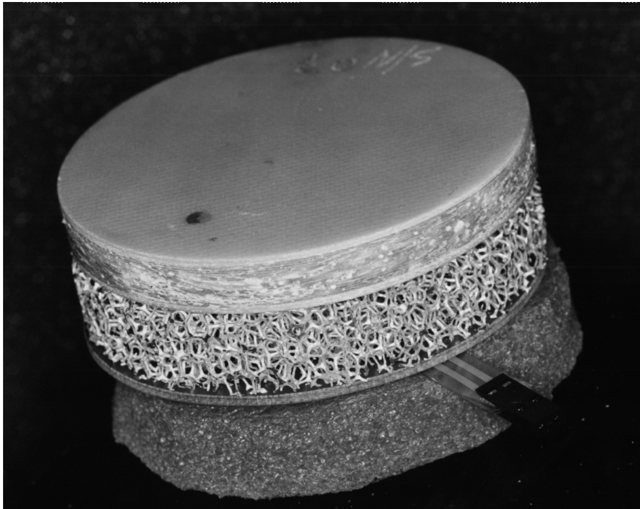
Figure D-8. Cross-section of COPV impact protector.
