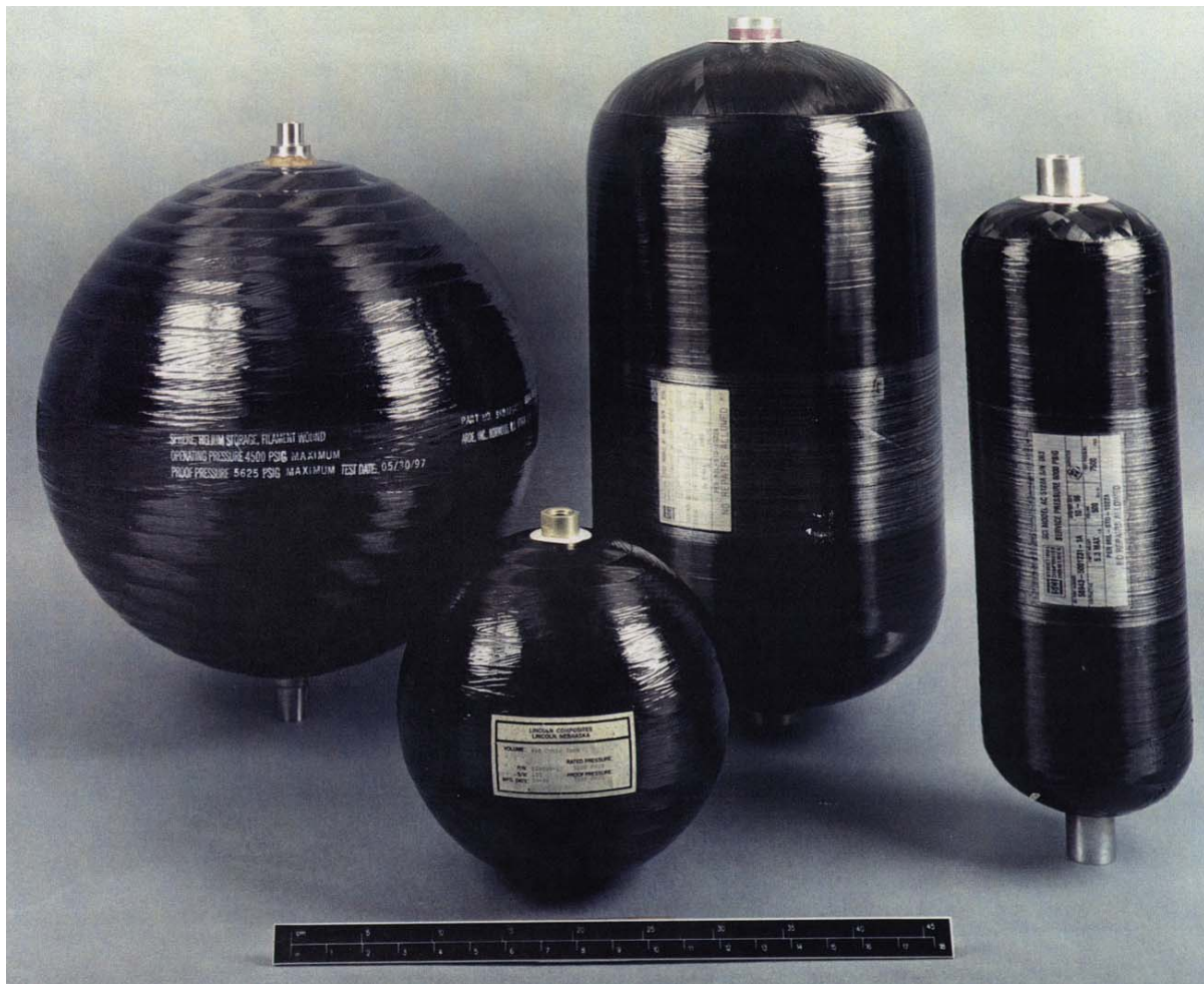
Figure B-1. Four types of flight qualified COPVs used as impact test specimens.
