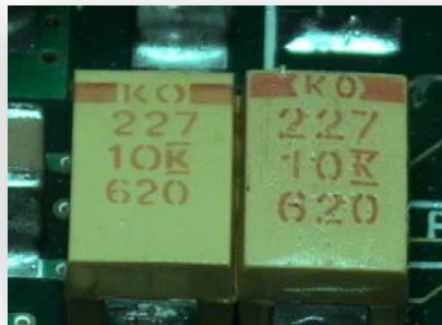
Marking slightly different on counterfeit part
