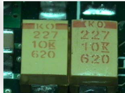
Marking slightly different on counterfeit part
