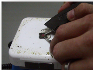
Counterfeiter removing die from part
