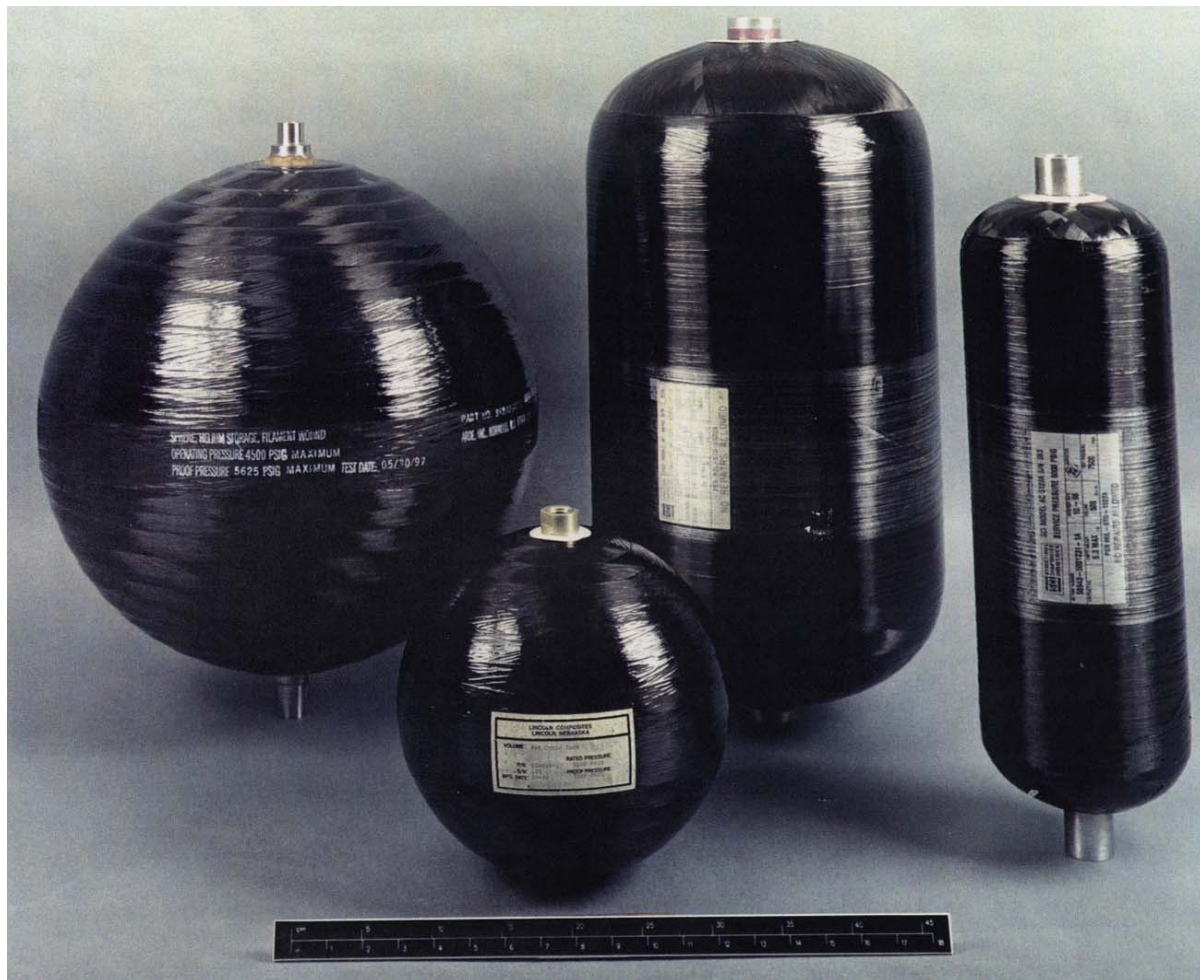
Figure C-1. Four types of flight-qualified COPVs used as impact test specimens.
