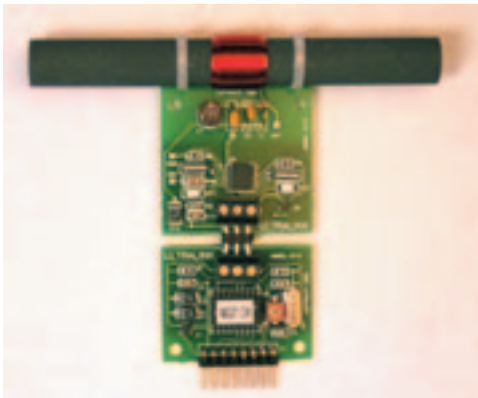
Figure 2.9. WWVB Receiver Circuit
