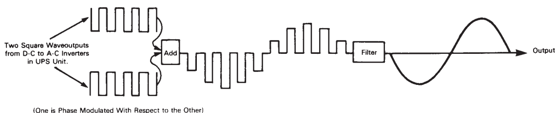
Figure 59. Static UPS with phase demodulated carrier: This partial schematic illustrates the principle used in some UPS hardware designs which sums two high-frequency waves. One is phase modulated at the desired output frequency (50, 60, or 400 Hz). A low-pass filter passes current at power frequencies, but rejects the inverter carrier frequency.
