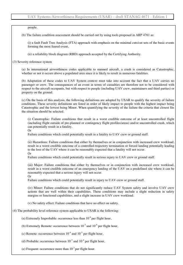
For systems and equipment used only in certain phases of flight (e.g., landing gear), a probability reference of "per flight" instead of "per flight hour" may be used at the discretion of the Certifying Authority (see FAR AC23.1309-1C).
