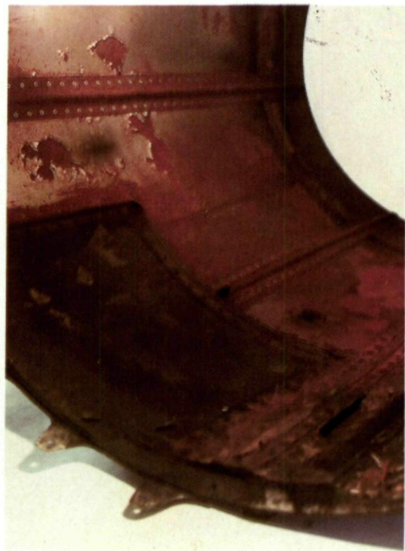
Fig. 7-2 Rusting in a jet pipe end cap liner following damage to its protective coating
