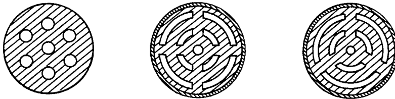
Figure 25.—Typical multiperforated grain shapes.
