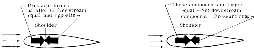
(b) Ideal fluid airfoil (no pressure drag).
