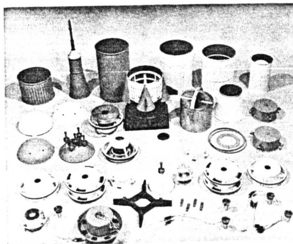
FIGURE 5.45.—Components of 1/40-scale model of Saturn V.
