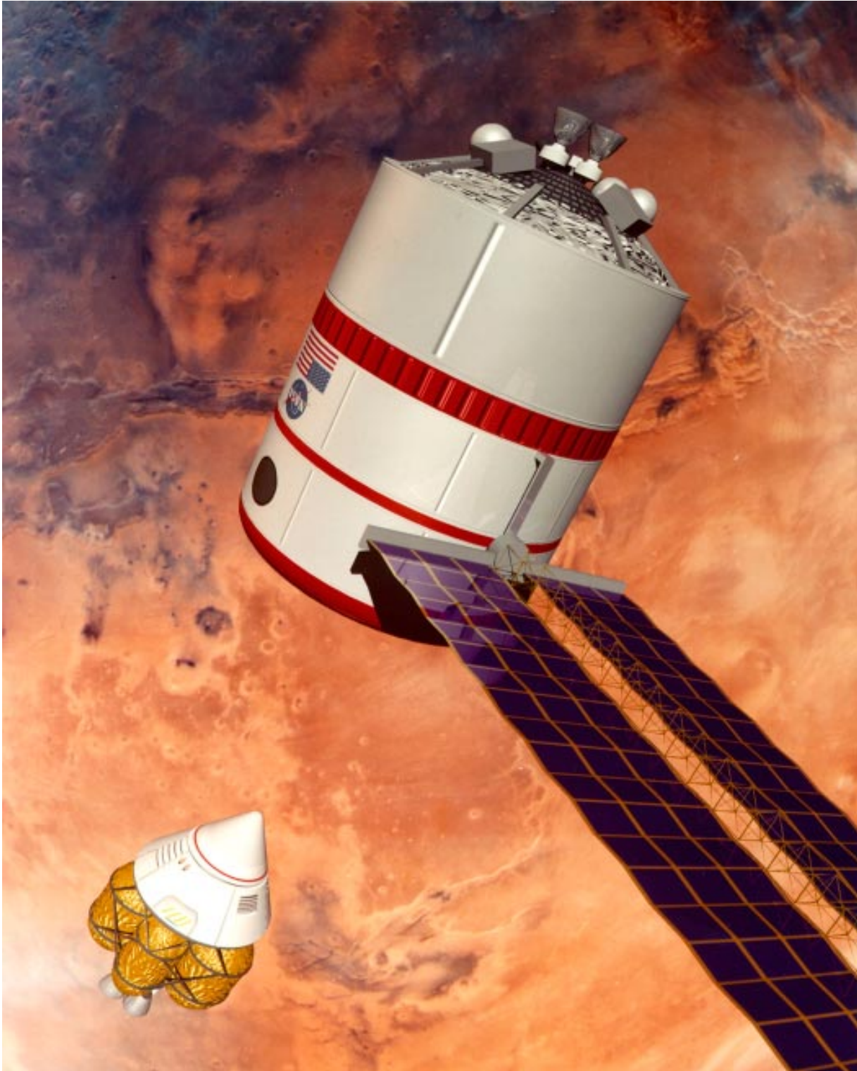
Figure 3-33 Solar array power source for interplanetary spacecraft.
