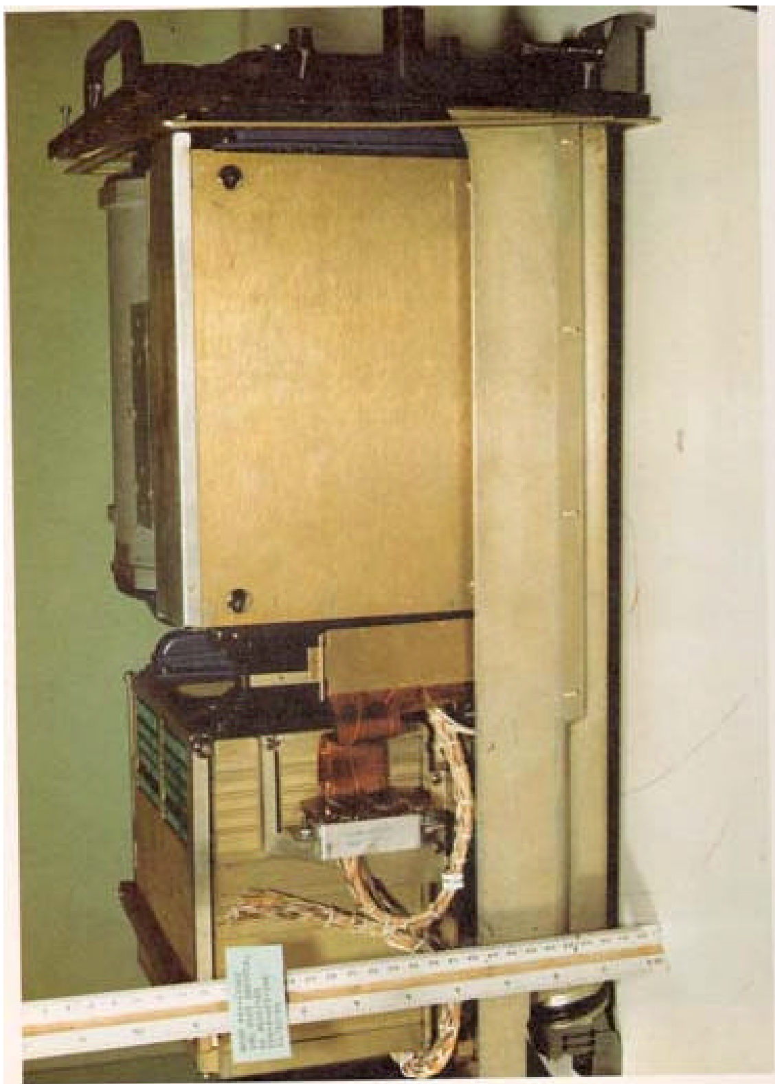
Figure 6-11.- Inertial measurement unit, internal view (pretest)
