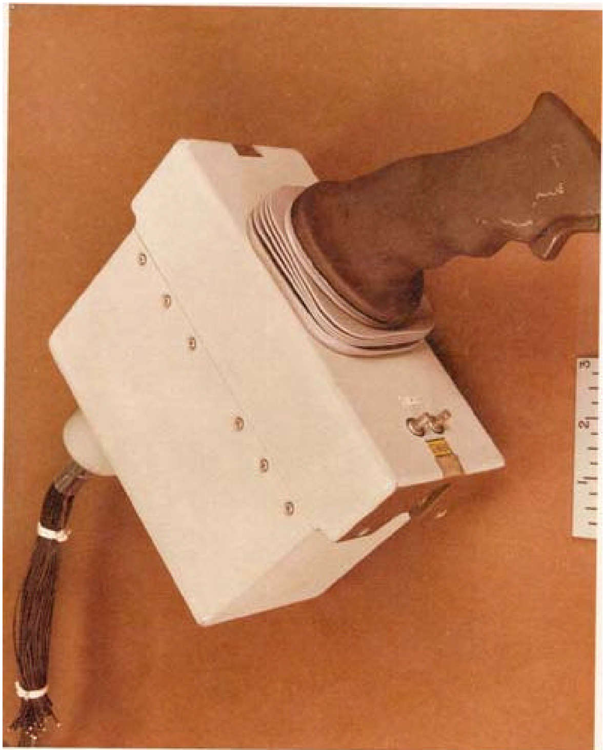
Figure 6-8 - Rotational controller (pretest).
