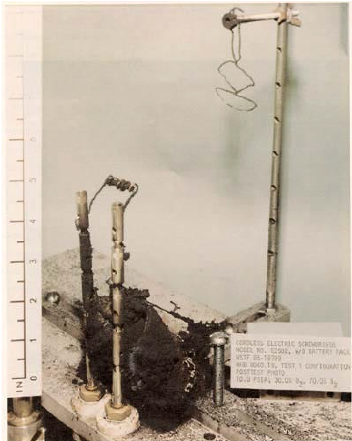
Figure 3-2.- Battery-powered screwdriver (post-test).
