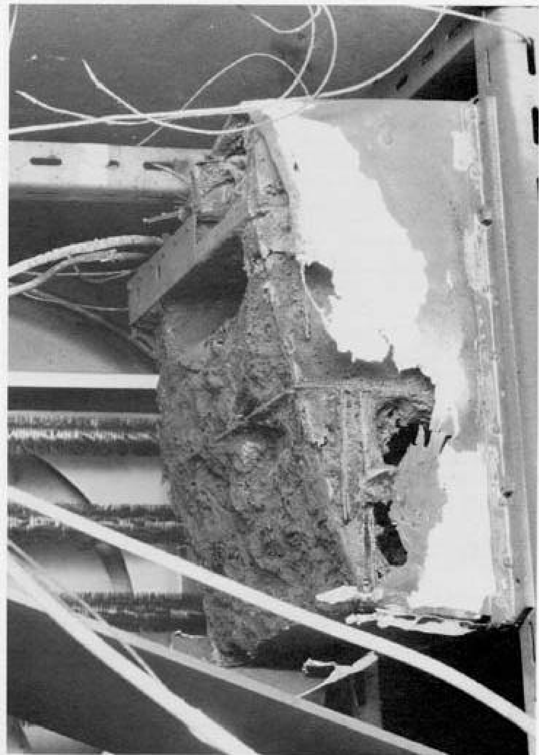
Figure 6-5 - Static inverter (post-test).
