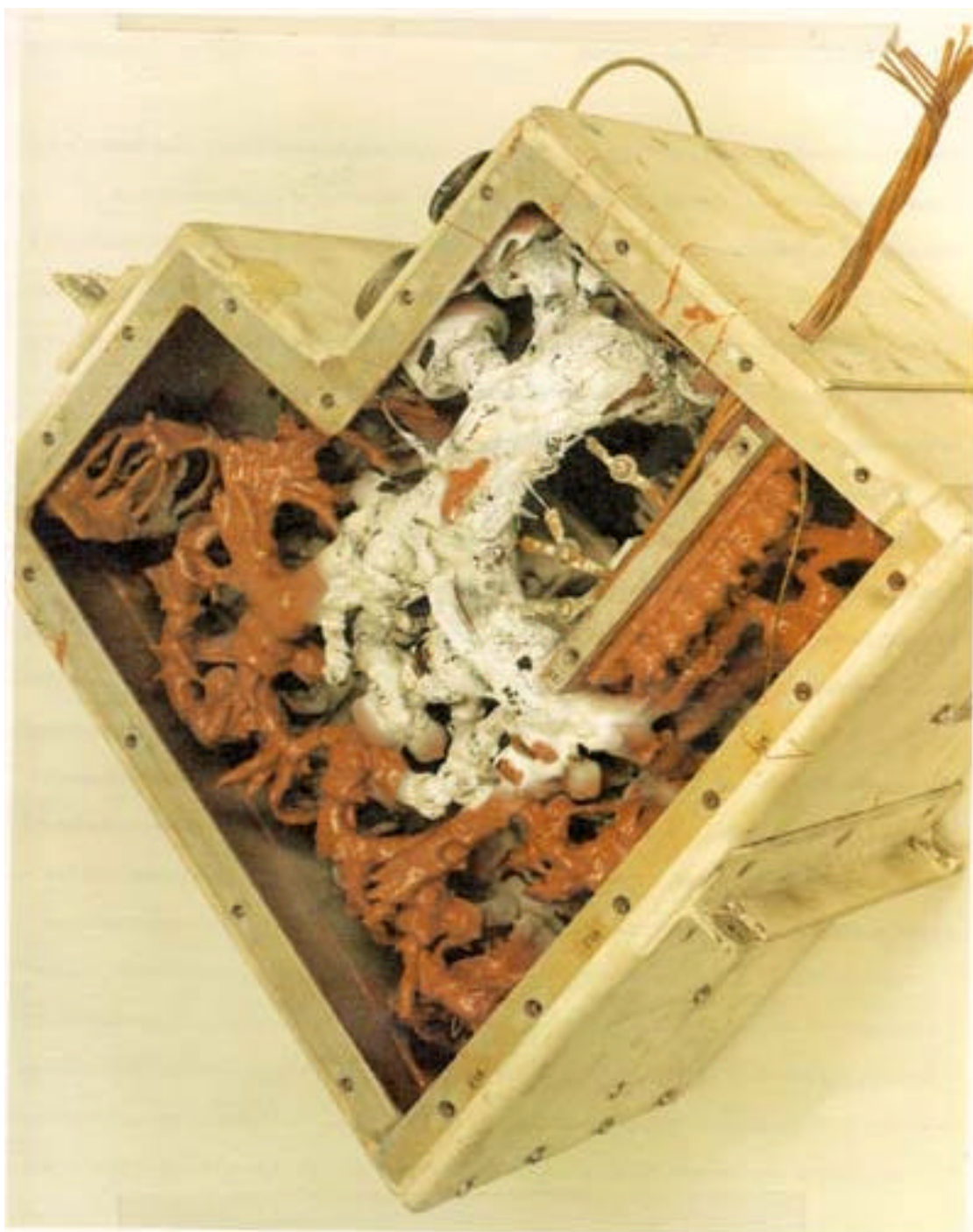
Figure 6-3. - Master events sequence controller (post-test).
