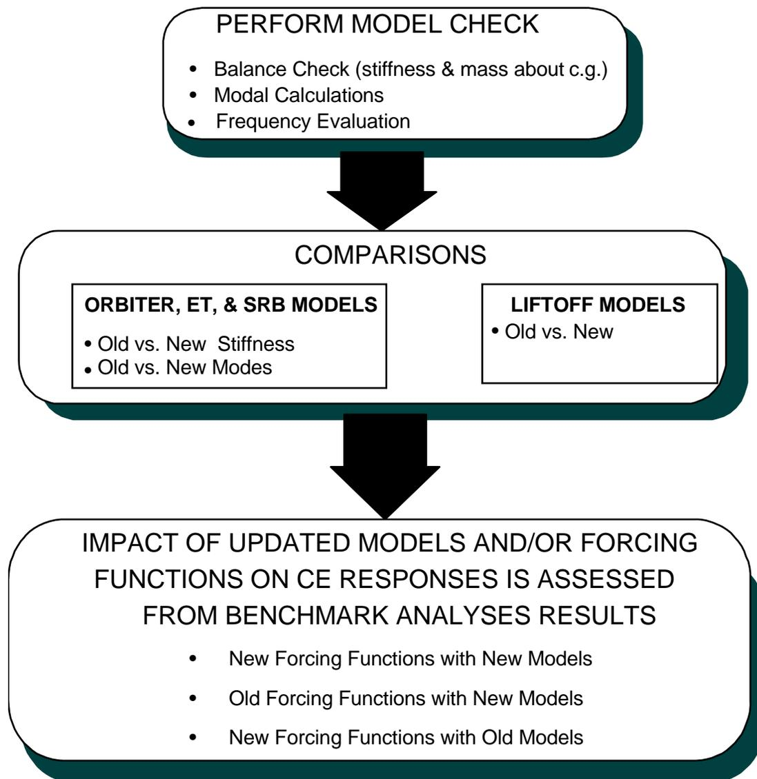
Figure 2.1-1.- SSV math model and forcing function evaluation.
