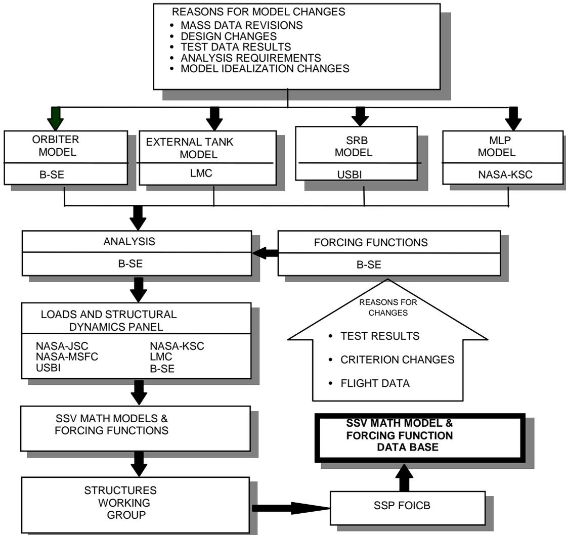
Figure 2.1-2.- SSV math model and forcing function configuration control.
