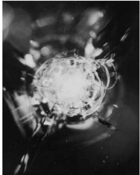
Figure A3. Nomarski image of laser-induced damage to uncoated, fused silica specimen. Magnification = 75x.
