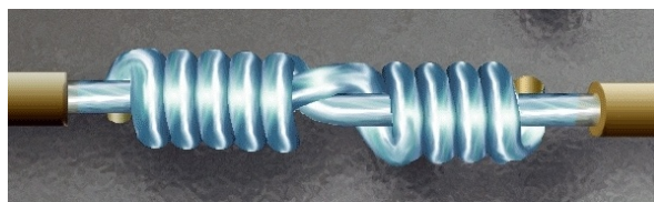
Figure 19-16. Completed Wrap for Western Union/Lineman Splice
