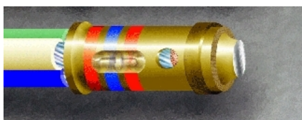
Figure 19-23. Contact Trimmed and Deburred
