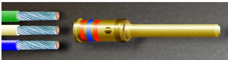
Figure 19-20. Stripped Wires Prior to Insertion
