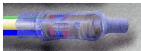
Figure 19-24. Contact Covered With Shrink Sleeving
