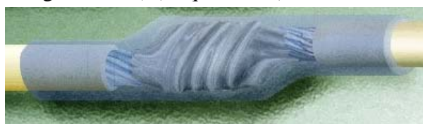
Figure 19-11. Sleeved Lash Splice
