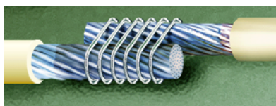
Figure 19-6. Lashing of Pre-Tinned Conductors
