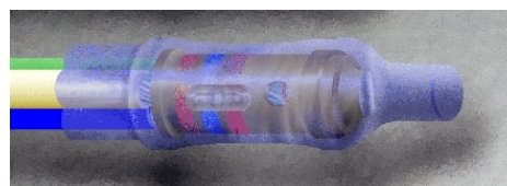
Figure 19-24. Contact Covered With Shrink Sleeving
