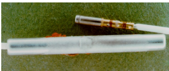
Figure 19-32. Crimped Contact Outside Junction Device
