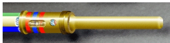
Figure 19-22. Wires Crimped Within Contact
