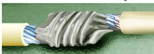
Figure 19-10. Soldered Lash Splice
