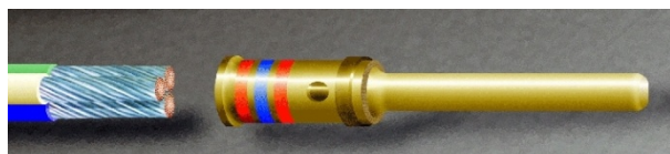
Figure 19-21. Stripped Wire Bundle Prior to Insertion
