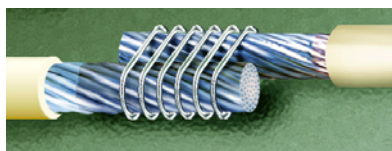
Figure 19-6. Lashing of Pre-Tinned Conductors
