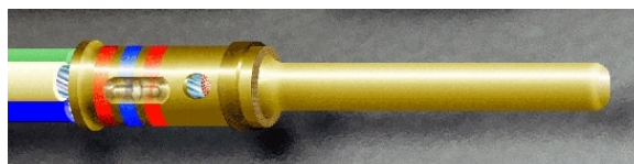
Figure 19-22. Wires Crimped Within Contact
