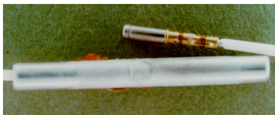
Figure 19-32. Crimped Contact Outside Junction Device
