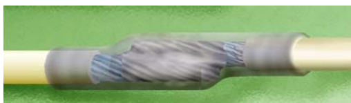
Figure 19-3. Sleeving over Soldered Connection
