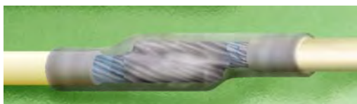
Figure 19-3. Sleeving over Soldered Connection
