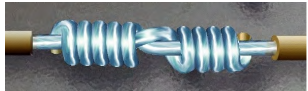
Figure 19-16. Completed Wrap for Western Union/Lineman Splice
