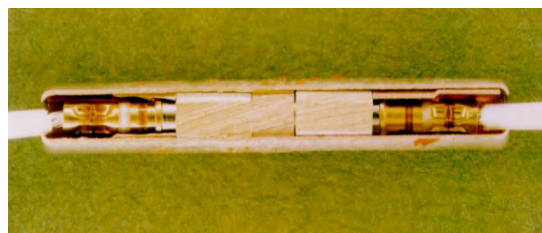
Figure 19-33. Crimped Contacts Inserted Into Junction Device
