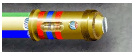
Figure 19-23. Contact Trimmed and Deburred
