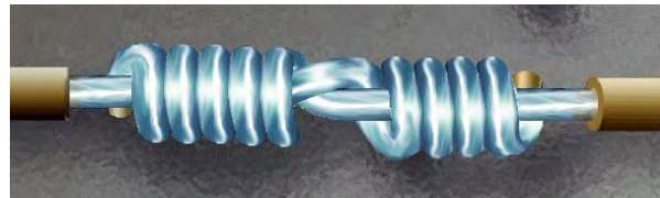
Figure 19-16. Completed Wrap for Western Union/Lineman Splice
