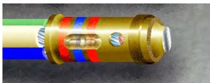
Figure 19-23. Contact Trimmed and Deburred
