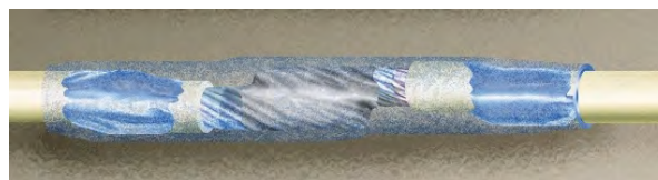
Figure 19-13. Fully Melted Solder Sleeve
