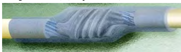
Figure 19-11. Sleeved Lash Splice
