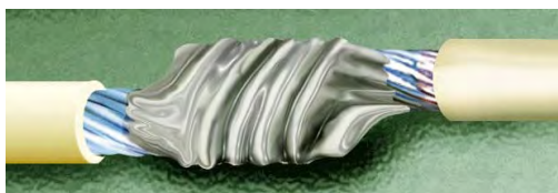
Figure 19-10. Soldered Lash Splice
