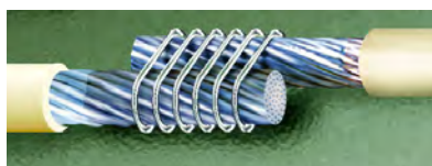
Figure 19-6. Lashing of Pre-Tinned Conductors
