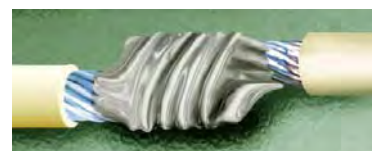
Figure 19-7. Soldered Connection
