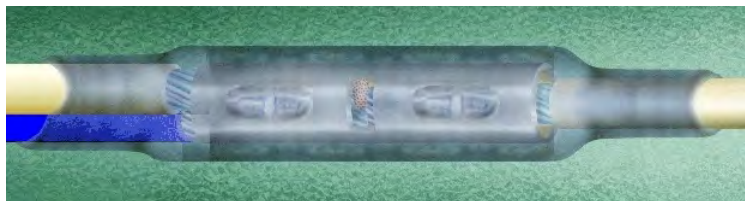
Figure 19-31. Butt Splice with Shrink Sleeving
