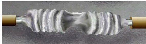
Figure 19-17. Soldered Western Union/Lineman Splice
