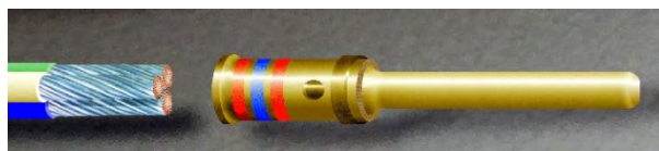
Figure 19-21. Stripped Wire Bundle Prior to Insertion
