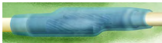
Figure 19-4. Double Sleeving over Soldered Connection
