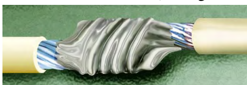
Figure 19-10. Soldered Lash Splice
