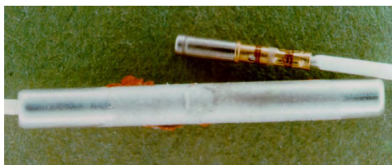
Figure 19-32. Crimped Contact Outside Junction Device
