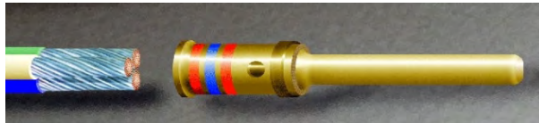
Figure 19-21. Stripped Wire Bundle Prior to Insertion
