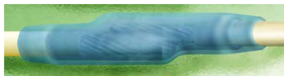
Figure 19-4. Double Sleeving over Soldered Connection
