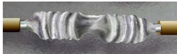
Figure 19-17. Soldered Western Union/Lineman Splice
