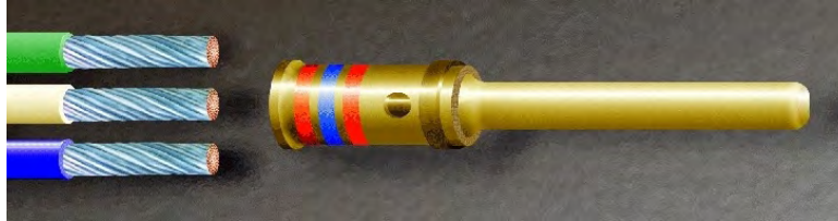
Figure 19-20. Stripped Wires Prior to Insertion
