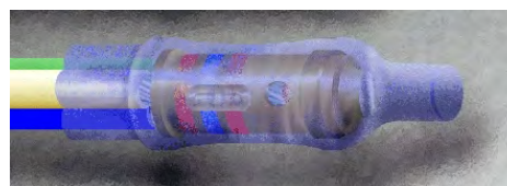
Figure 19-24. Contact Covered With Shrink Sleeving
