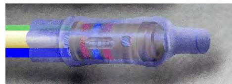
Figure 19-24. Contact Covered With Shrink Sleeving
