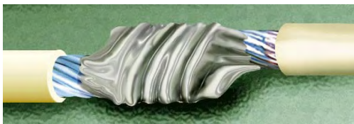
Figure 19-10. Soldered Lash Splice
