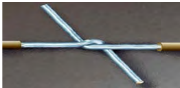
Figure 19-15. Initial Wrap for Western Union/Lineman Splice
