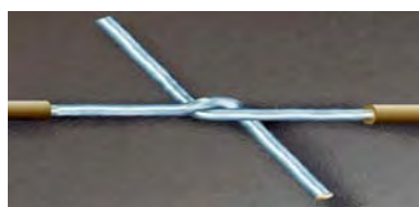
Figure 19-15. Initial Wrap for Western Union/Lineman Splice
