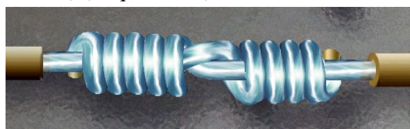
Figure 19-16. Completed Wrap for Western Union/Lineman Splice
