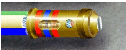
Figure 19-23. Contact Trimmed and Deburred
