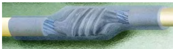
Figure 19-11. Sleeved Lash Splice
