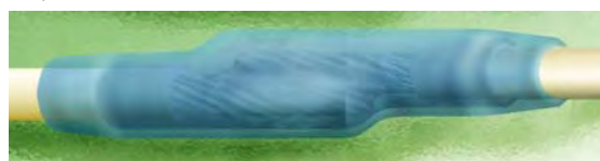
Figure 19-4. Double Sleeving over Soldered Connection
