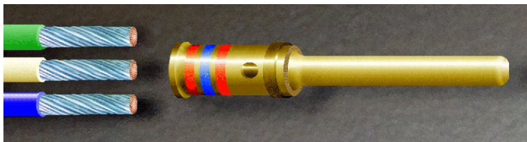
Figure 19-20. Stripped Wires Prior to Insertion
