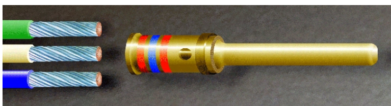
Figure 19-20. Stripped Wires Prior to Insertion
