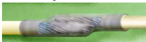
Figure 19-3. Sleeving over Soldered Connection
