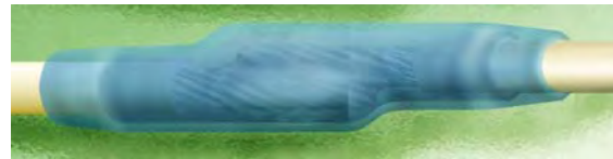
Figure 19-4. Double Sleeving over Soldered Connection
