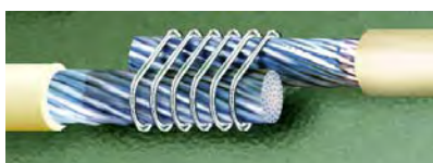
Figure 19-6. Lashing of Pre-Tinned Conductors
