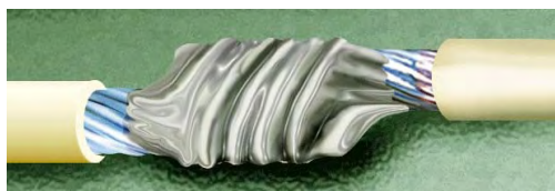
Figure 19-10. Soldered Lash Splice
