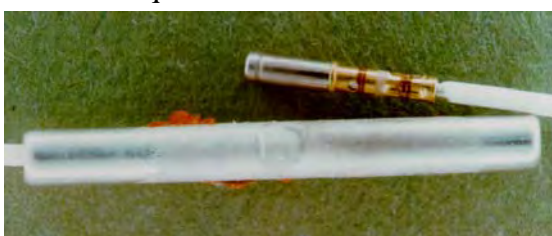
Figure 19-32. Crimped Contact Outside Junction Device
