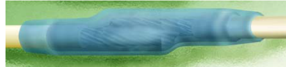
Figure 19-5. Double Sleeving over Soldered Connection
