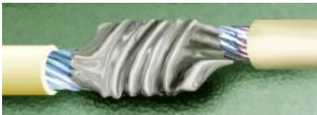
Figure 19-11. Soldered Lash Splice
