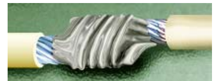
Figure 19-8. Soldered Connection
