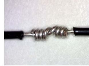
Figure 19-17. Completed Wrap for Western Union/Lineman Splice
