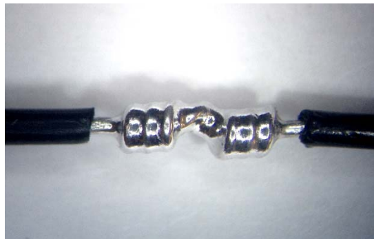
Figure 19-18. Soldered Western Union/Lineman Splice
