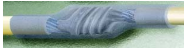
Figure 19-12 Sleeved Lash Splice
