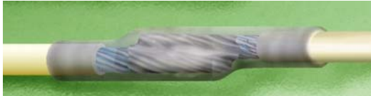
Figure 19-4. Sleeving over Soldered Connection
