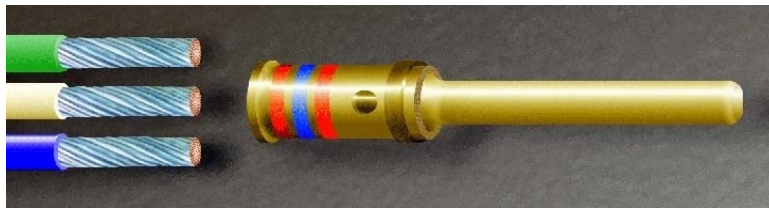
Figure 19-21. Stripped Wires Prior to Insertion
