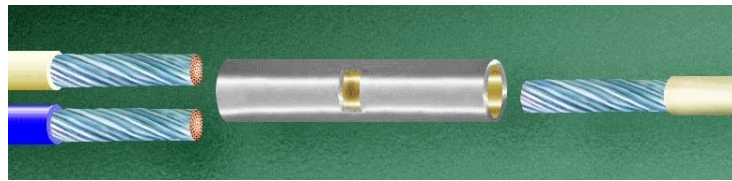
Figure 19-29. Butt Splice Prior to Wire Insertion
