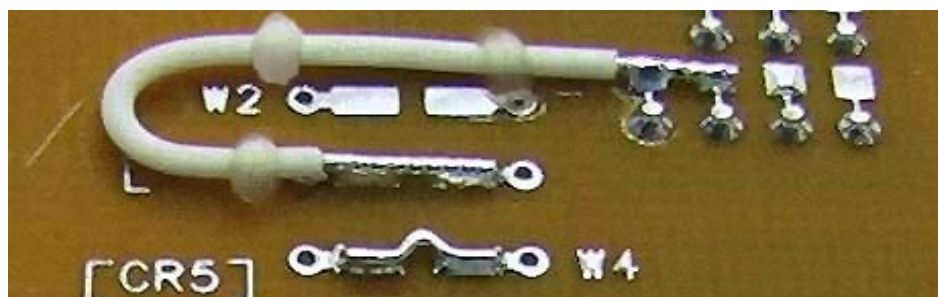
Figure 9-2. Single Wire Staking
