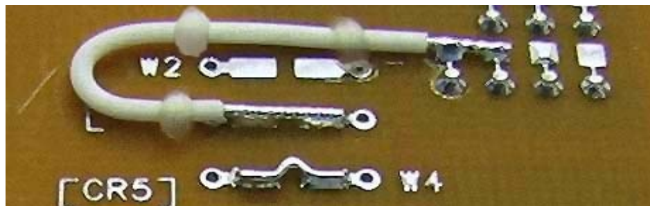
Figure 9-2. Single Wire Staking
