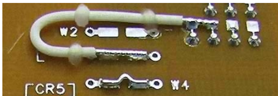
Figure 9-8: Single Wire Staking
