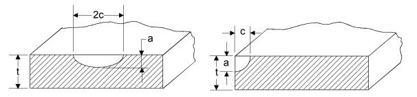
FIGURE 2. Standard Crack Geometries
