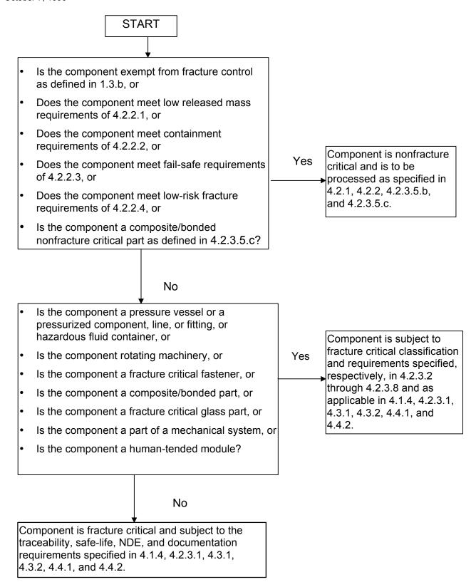
FIGURE 1. Fracture Control Classification/Processing of Payload Components
