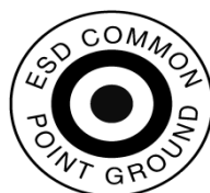
Figure 8-3: ESD Common Point Ground Symbol
