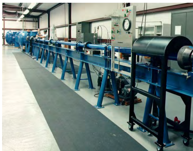
Figure 4.6-3. NASA JSC-White Sands Test Facility two-stage LGG.
