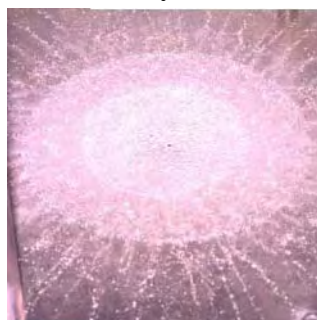
Figure 4.6-7. Rear wall after impact.
