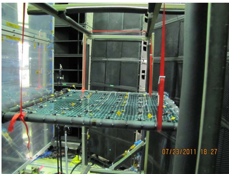
Figure 8—A Microphone Array Used to Obtain Spatial Mapping of the SPL in Various Slices of the Test Field
