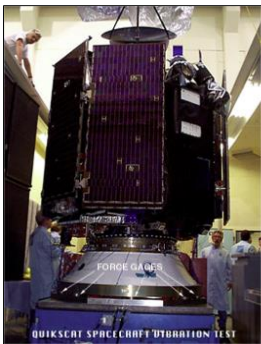
Figure 44—Spacecraft Vibration Test
