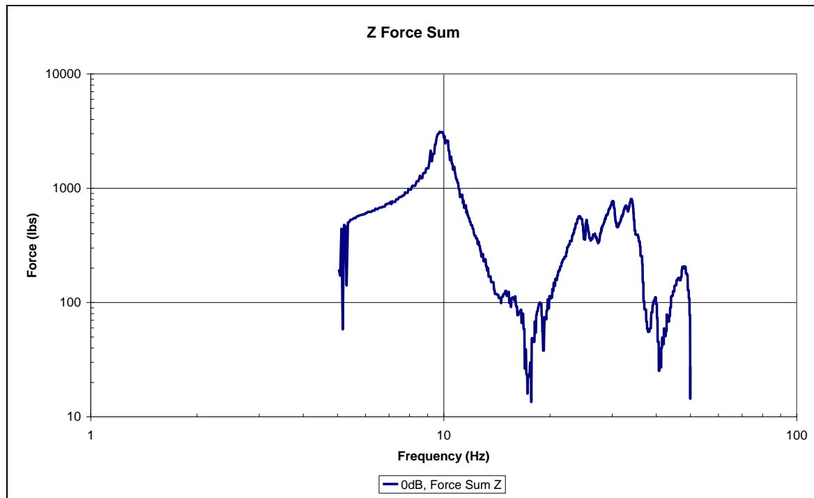
Figure 35—Z-Axis Force Sum for 0-dB Sine Run
