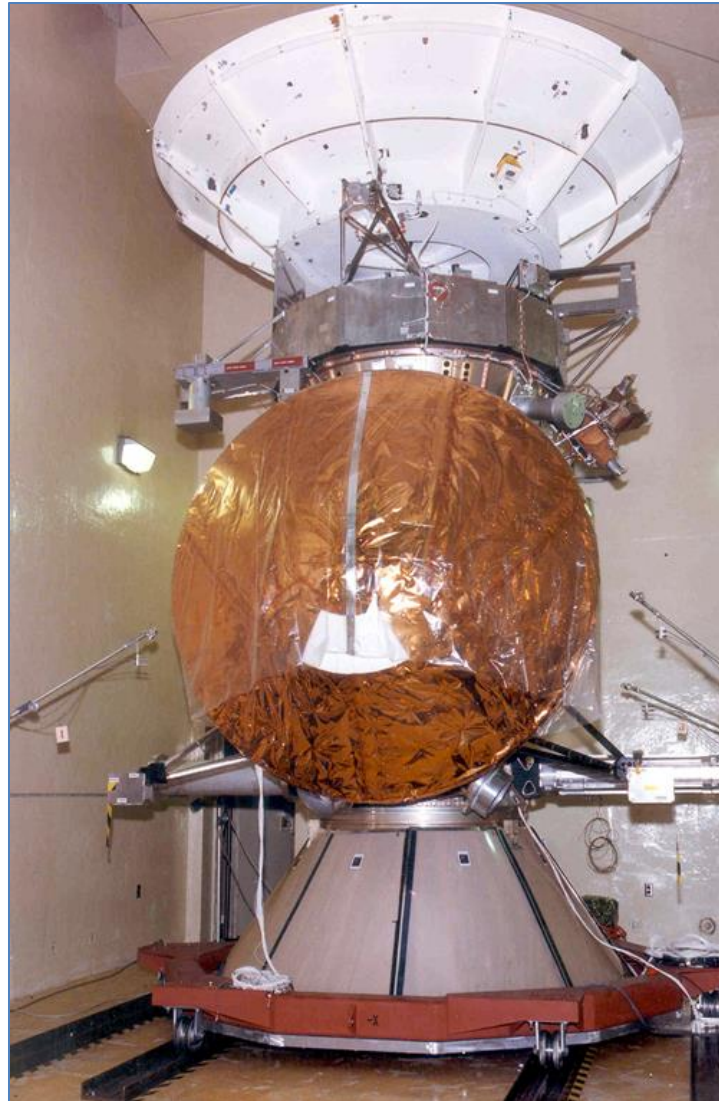
Figure 7—Cassini DTM Spacecraft in JPL Acoustic Chamber
