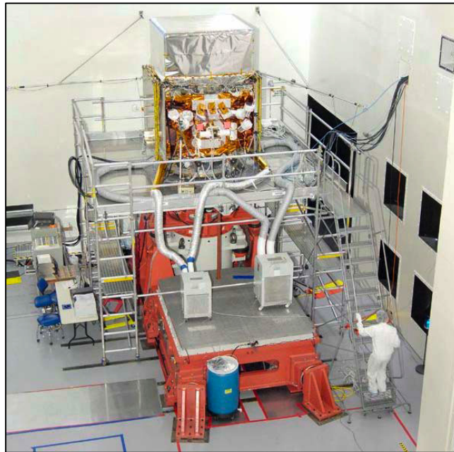
Figure 21—GLAST Spacecraft Sine Vibration Test
