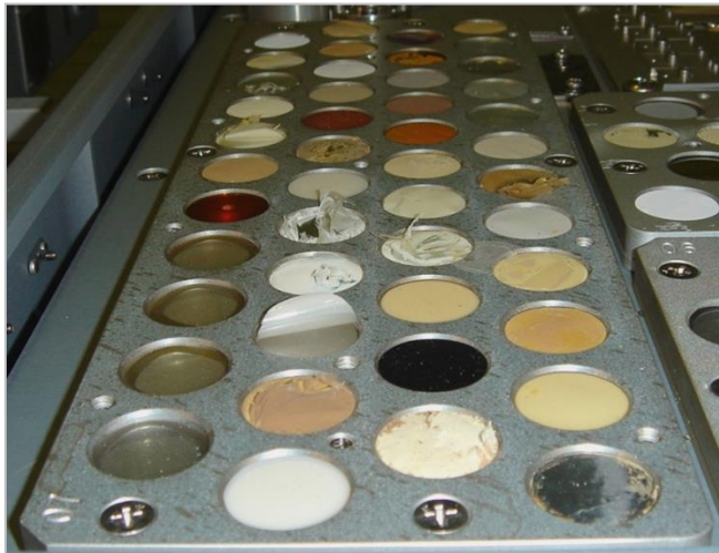
Figure 33—PEACE Polymers Experiment Tray in the NASA LaRC Clean Room during Post-Flight Retrieval Examination
