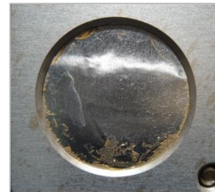
(c) Completely Eroded PBI (2-E5-35)
