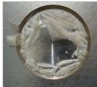
(b) Partially Eroded PMMA (2-E5-16)
