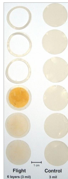
Post-flight photograph of individual sample layers. Layers were separated for weighing. (Mass loss Situation 2)
