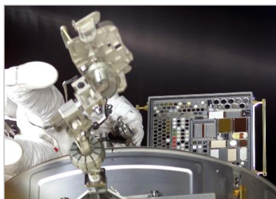
(b) Securing the PEC in the Opened Position, Exposing the Samples to Space
