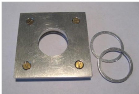
Figure 57—Sample Holder for Optical and Thermal Measurements
