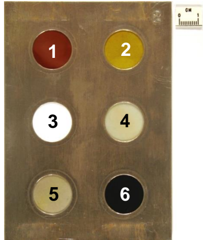
Figure 45—Sample Holder with Six Polymer Samples
