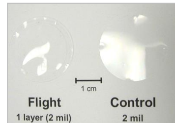
Post-flight photograph of sample single layer (Mass loss Situation 1)
