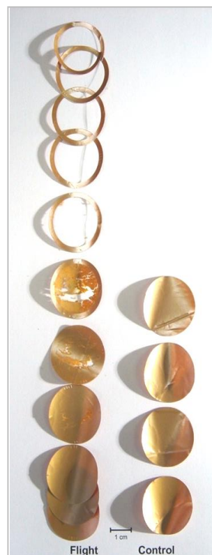
Post-flight photograph of individual sample layers (11 flight; 4 control). Layers were separated for weighing postflight. (Mass loss Situation 2)
