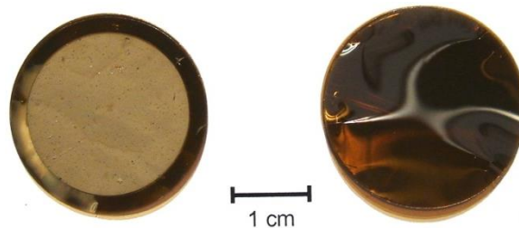
(a) Flight Sample Stack (2-E5-32) (b) Control Sample Stack
