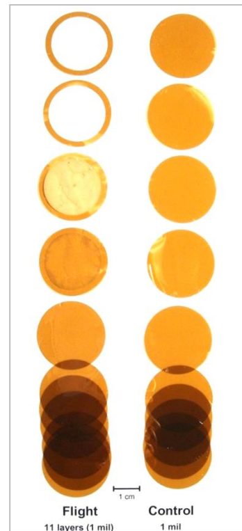
Post-flight photograph of individual sample layers (11 flight; 10 control). Layers were separated for weighing. (Mass loss Situation 1)
