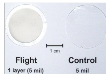
Post-flight photograph of stacked sample layers. Sample layers could not be separated for weighing. (Mass loss Situation 1)
