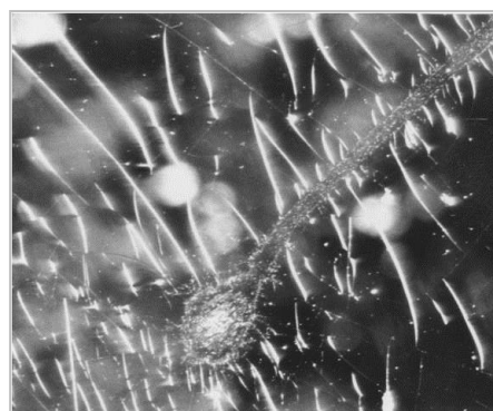
(b) Post-Flight with Mud-Tile Cracking Observed
