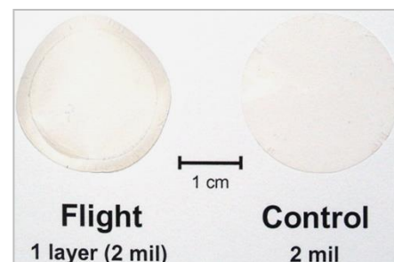
Post-flight photograph of sample single layer (Mass loss Situation 1)
