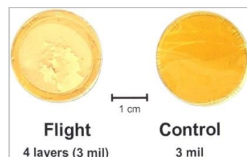
Post-flight photograph of stacked sample layers. Sample layers could not be separated for weighing. (Mass loss Situation 3)
