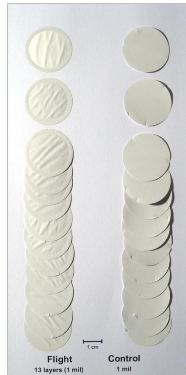
Post-flight photograph of individual sample layers. Layers were separated for weighing. (Mass loss Situation 1)
