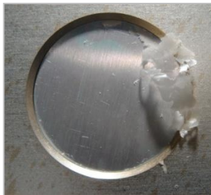
(a) Partially Eroded PE (2-E5-9)
