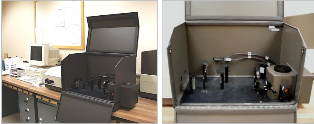
Figure 58—Perkin Elmer Lambda 19 Spectrophotometer with Closeup of Integrating Sphere
