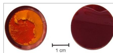
Post-flight photograph of stacked sample layers. Sample layers could not be separated for weighing. (Mass loss Situation 3)
