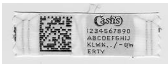
FIGURE 22. Cloth Label Produced Using Fabric Weaving Technique
