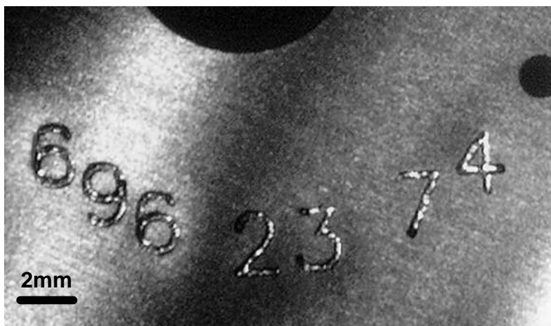
FIGURE 8. Direct Part Marking Using LENS. A Molybdenum Disk Was Marked With Stainless Steel Raised Lettering.
