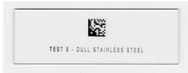
FIGURE 35. Stainless Steel Marking Applied To Glass Slide Using LIVD Process
