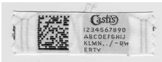
FIGURE 22. Cloth Label Produced Using Fabric Weaving Technique
